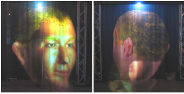
Figure 2. The support for dual-sided projection allows two independent images to be projected on each side, such that a 3D application can render two interactive views for a pseudo-3D effect.
