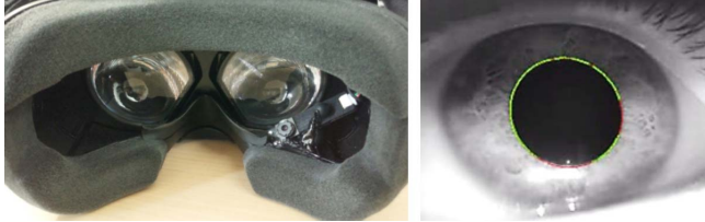
Fig. 1. Images showing the HTC Vive with integrated pupil labs tracker (left) and a screenshot from the video stream with the tracked pupil ellipse (right), which is a customized version of open-source tracking software [14].
