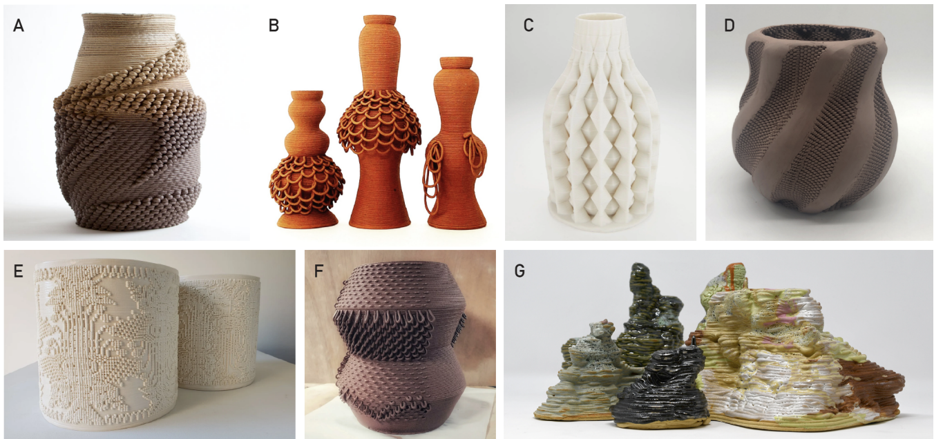
Figure 3: 3D printed clay artifacts showcasing a variety of form and textural qualities. A) Design studio Emerging Objects creates texture effects that form a global pattern [63]. B) Designer Virginia San Fratello plays with the material properties of clay to form drooping loops on organic looking forms [67]. C) Bryan Czibez stacks layers of intersecting paths defined parametrically to create sharp geometric forms [21]. D) Monica Silva Lovato uses a clay-specific slicer to create more stable structures and surface texture [28]. E) Timea Tihanyi prints porcelain with a fine nozzle to create intricate textures akin to woven patterns [83]. F) Bold Design Studio defines precise geometrical zones where surface texture is applied on the vessel [14]. G) Raina Lee creates organic forms by stacking hand-drawn lines [30].
