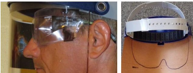
Figure 3: Left: Fresnel glasses with a head-mounted image (left eye image removed for clarity). Right: The measured visible screen area of the glasses prototype.
