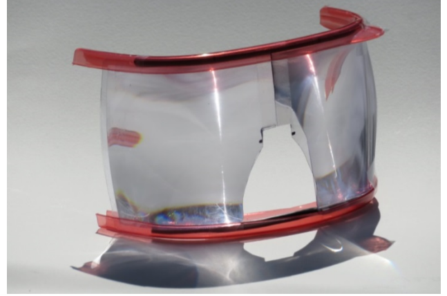
Figure 2. Super-wide-FOV curved Fresnel mask prototype
