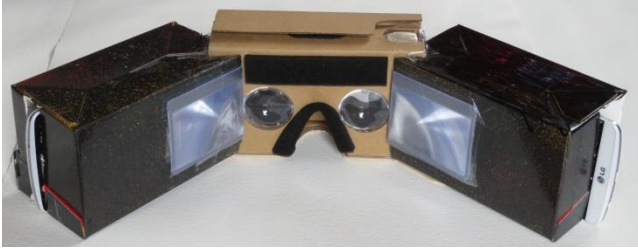
Figure 1. Wide-FOV peripheral extension screens (lenses and smartphones) added to a Google Cardboard.
