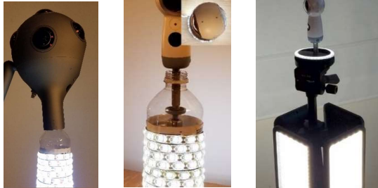
Figure 2: LEDs behind a Nokia Ozo camera (left). LEDs below the Samsung Gear 360 camera (middle), and the same seen from up (middle, insert). A bright LED panel light box below the Samsung Gear 360 camera (right).
