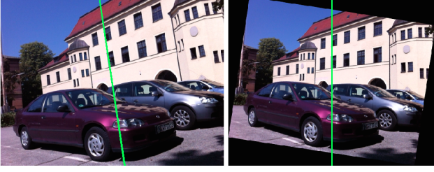
Figure 2: The gravity vector (green) may be obtained from sensor measurements on common smartphone devices. By aligning the gravity vector to the known gravity direction [0, -1, 0]^T , we remove 2 d.o.f. from the unknown rotation to create a simplified absolute pose method.
