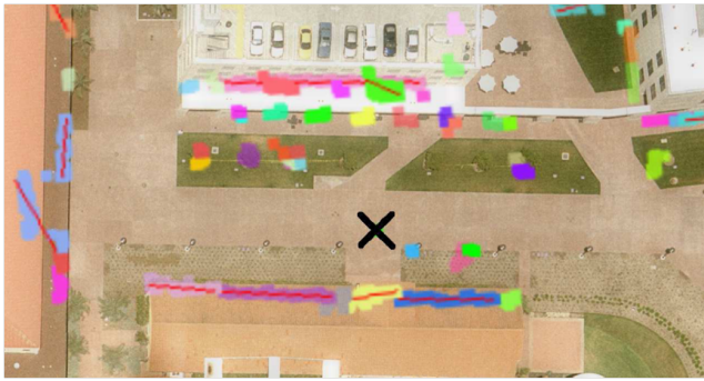
Figure 2: Planes detected using a laser rangefinder are overlaid on an aerial photograph. Each color represents one cluster of points corresponding to a plane. The cross marks the point of capture. Figure from Wither et al. [26].
