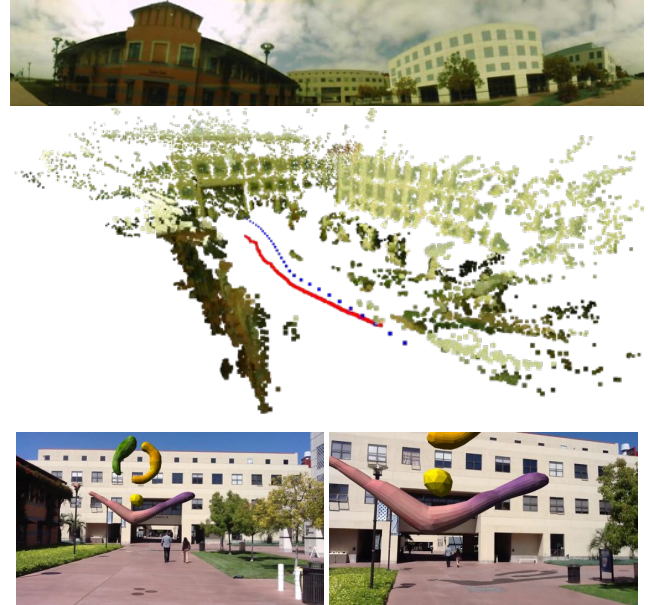
Figure 1: Overview of system operation. Top : Panorama from a thirty second video taken with a handheld omnidirectional camera while walking. Middle : Point cloud reconstruction produced in under fifteen minutes (densified for better visualization [8]). The blue points indicate panorama locations. Bottom : Two frames from an iPad video tracked in real-time with situated 3D graphics added. The camera track is plotted in red in the middle image.
