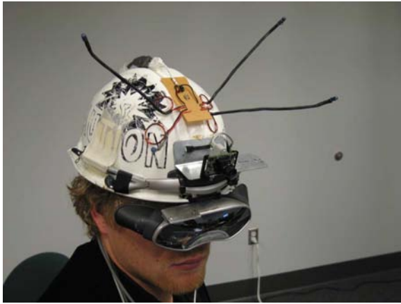
Figure 6: The HMD we in our study. The four arms support infrared LEDs used for 6DOF tracking.
