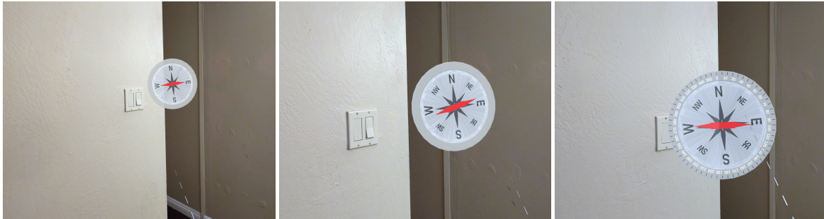
Figure 1: Images of the Level-of-Detail AR mechanism applied to a compass application. The level of detail, such as the points on the compass, adjusts as the visual angle changes due to a decreasing distance between the user and the object. The image on the left shows the compass at the farthest distance from the user, resulting in the cardinal directions being included in the display and the non-cardinal directions being excluded from the display. The image in the center, which shows the compass at a smaller distance from the user, includes both the cardinal and non-cardinal directions in the display but excludes the degrees and their associated markings. The image on the right, in which the compass is the closest to the user, shows all levels of detail for the compass application including the display of cardinal directions, non-cardinal directions, degrees, and degree markings.
