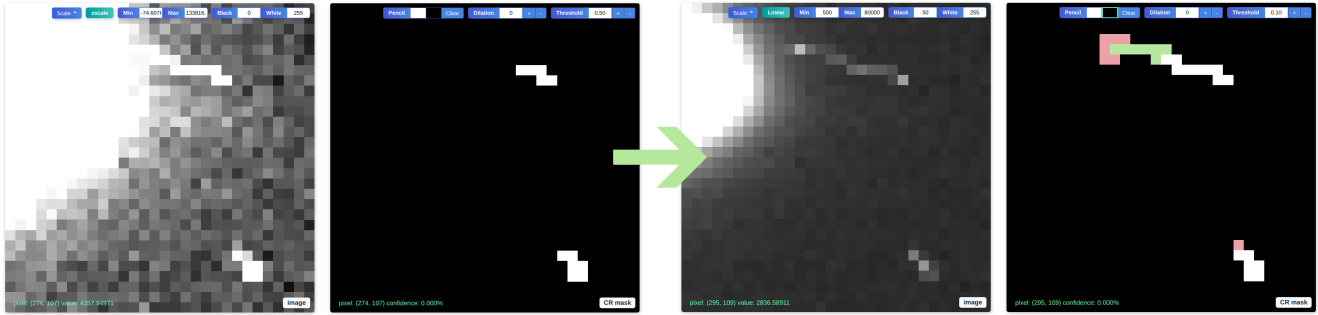
Figure 2. When the model or the default threshold does not produce ideal results (left), the user can adjust the HDR image mapping for better visualization, at the same time edit the mask interactively (right). The probability threshold and morphological dilation allow for global mask manipulation, while the pencil tool allows pixel-level mask editing. Pixels that are manually added/deleted by the user are marked in green or red, which will override the global manipulations.
