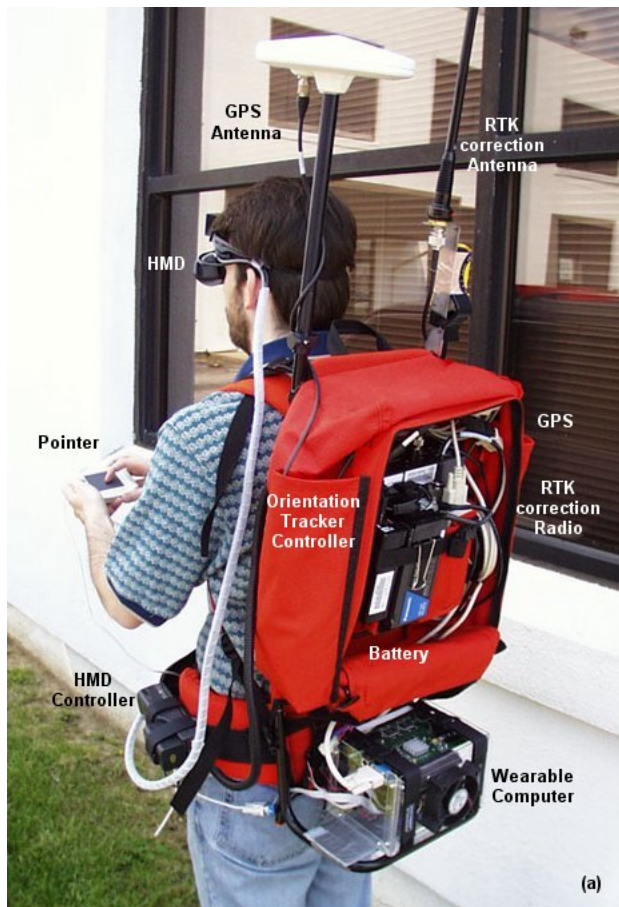
Figure 1. Backpack based wearable augmented reality systems. (a) NRL system. (b) Columbia system.
