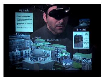
Figure 1. View management in augmented reality testbed (imaged through a tracked, see-through, head-worn display).
