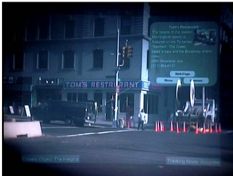
Figure 6: Image taken directly through an optical see-through head-worn display of restaurant and related popup information
