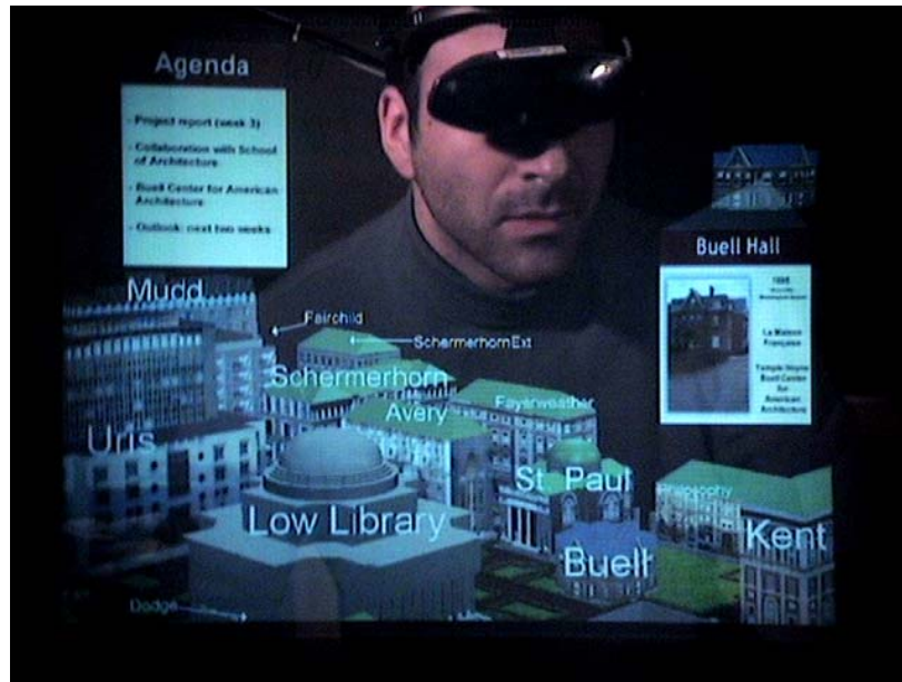
Figure 1. View management in augmented reality (imaged through a tracked, see-through, head-worn display).
