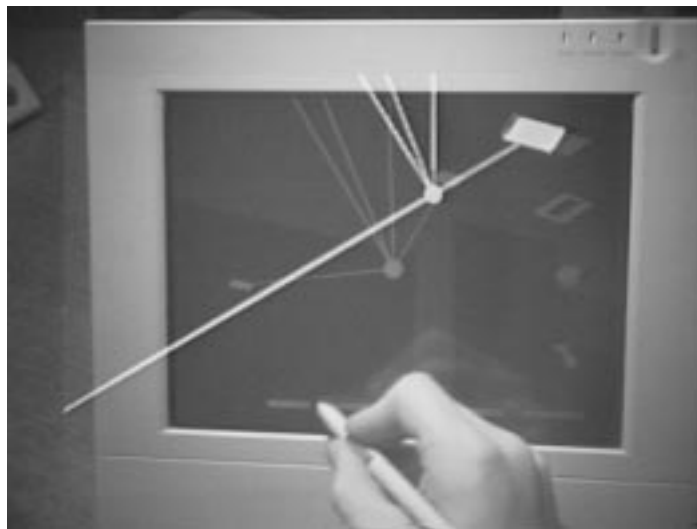
Figure 5: A simple interactive search mechanism creates 3D leader lines emanating from the tracked display to objects satisfying the query.
