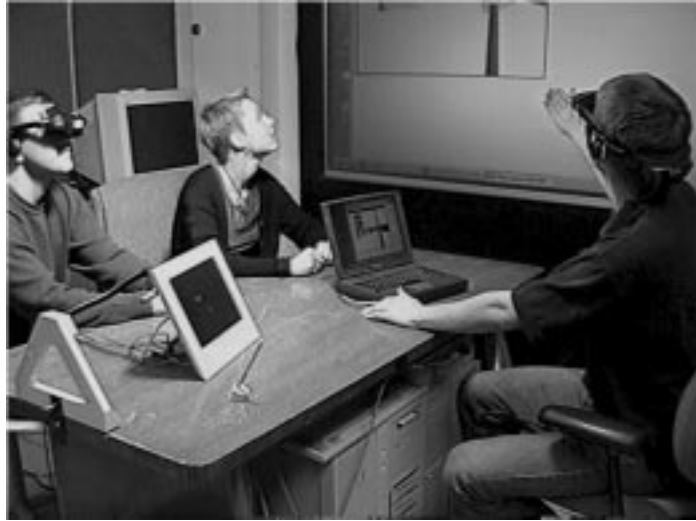
Figure 1: A meeting situation using EMMIE. Two users wear tracked see-through head-worn displays, one of whom has also brought in his own laptop. The laptop and a stylus-based display propped up on the desk are also tracked. All users can see a wall-sized projection display. The triangular source for one tracker is mounted at the left of the table; additional ceiling-mounted trackers are not visible here.
