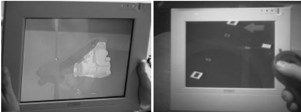
Figure 4: The same display tablet can serve as physical magic lens and magic mirror. In the left picture a user not wearing a HMD is looking through the magic lens at a 3D CAD object. In the right picture a user wearing a HMD has just dragged a virtual image slide in front of the mirror for further inspection.
