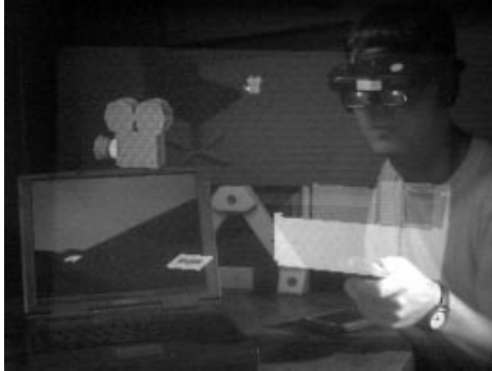
Figure 2: A user manipulates a 3D model with an optically tracked hand-held pointer. Other virtual objects shown include simple iconic 3D representations of applications (e.g., a “movie projector” that can play videos) and data objects (e.g., “slides” that represent still images).
