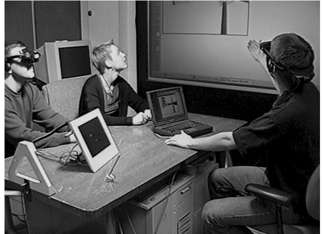
Figure 1. A meeting scenario using EMMIE. Two users wear tracked see-through head-worn displays, one of whom has also brought in his own laptop. The laptop and a stylus-based display propped up on the desk are also tracked, using sensors attached to their backs. All users can see a wall-sized projection display. The triangular source for one tracker is mounted at the left of the table; additional ceiling-mounted trackers are not visible here.
