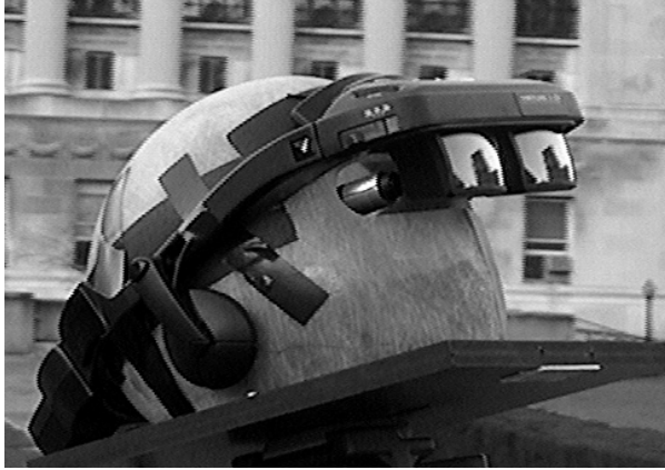
Figure 8. The dummy head used to capture images through our headworn display. A camera in the right eye socket captures what a user wearing the display would see.
