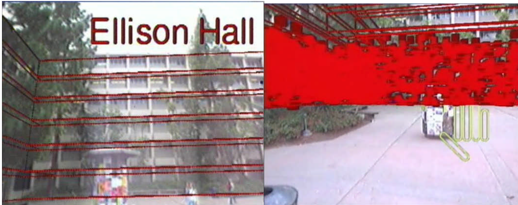
Figure 2: Left: AR-view of one of the two buildings that we built models for. Right: visualization of spots with "insufficient wireless" signal strength. The density of the data prohibits making out differences in the data intensity.
