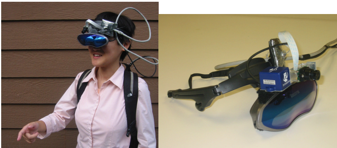
Figure 1: Left: a user wearing our system. Right: the head-worn display with the tracker attached.
