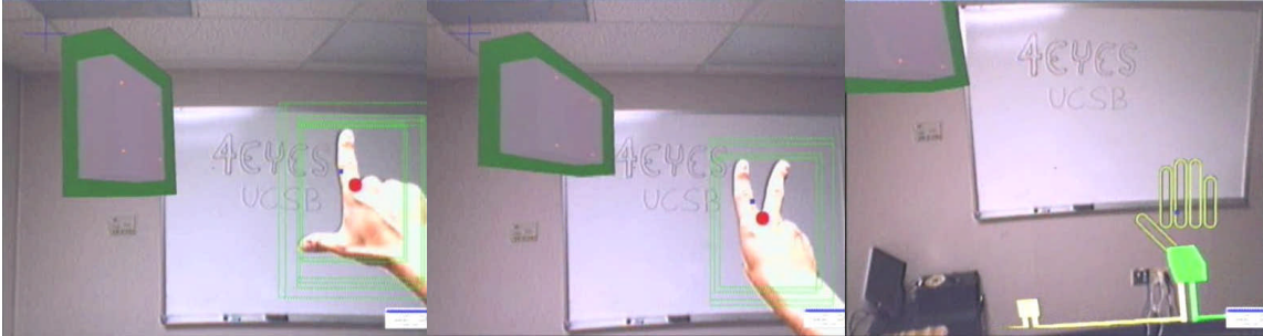
Figure 6: Resizing an object with gestures. The left picture shows the user’s hand in the ‘lock’ posture from which on hand location changes rescale the virtual object (the gray box with a green selection frame around it). In the middle picture, the user performs the ‘release’ posture, which decouples hand movements and object scale again. The right picture shows the placement of the virtual object in the left upper corner and representations for power and networking equipment near the floor.
