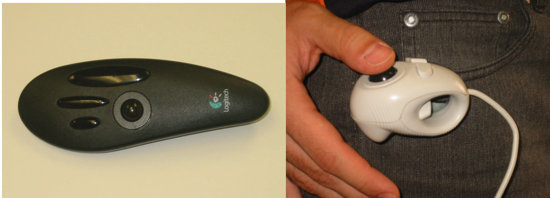
Figure 8: Our two favorite devices to provide one-dimensional input to our system, a wireless handheld trackball and a trackball that can be worn similar to a ring. Here it is attached to the user's pants with a Velcro strip.
