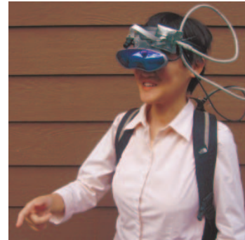
Figure 1: Our mobile user interface in action. All hardware components aside from display, camera, and microphone are in the backpack.
