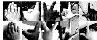
Figure 4: Two examples each of the five hand postures that are recognized, shown in the minimum resolution required for recognition, 25x25 pixels, some with a distorted aspect ratio for recognition performance reasons.
