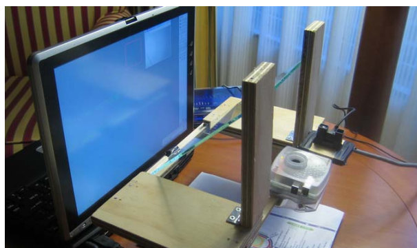
Figure 1. The POLAR system. The prototype AR setup uses a laptop, a custom-made foldable mount, a beam splitter (half-silvered mirror), a camera and an IR rangefinder.
