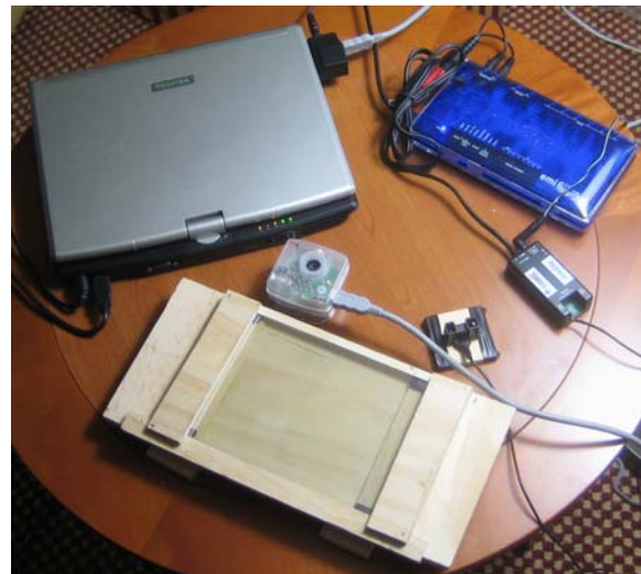
Figure 4. The POLAR system components in folded state. Clockwise from top left: Laptop, external soundcard (allows laptop to connect to the A/D converter's MIDI interface over USB), A/D converter with MIDI interface, IR rangefinder, folded mount with stored half-silvered mirror, and firewire camera. The external sound card and A/D converter will be replaced by a custom USB-based distance sensing module, about the size of the camera.
