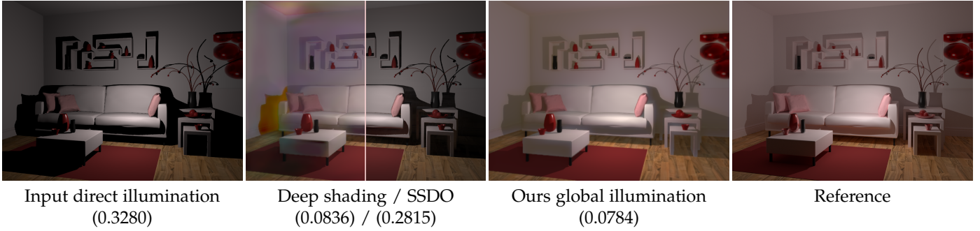
Fig. 1. Our method can predict high-quality global illumination with a resolution of 1024 \times 768 from direct illumination and auxiliary features such as normals and 3D positions. Our method runs at real-time framerates (45.3 FPS in this case) and generates much more plausible results compared with deep shading [1] and screen space directional occlusion [2]. The numbers above indicate the differences to the reference using the 1-SSIM metric.
