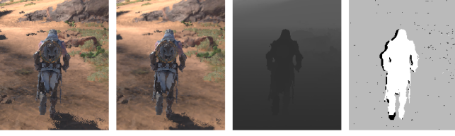
Fig. 7. The inputs of shading correction network (SCN). Images from left to right are: the output of GAE module \bar{I}_{t+\alpha}^{\text{GAE}} , the backward warped result I_{t-1 \rightarrow t+\alpha}^w from frame t-1 using motion vectors, the generated depth buffer \bar{D}_{t+\alpha} , and the input mask M_t^{\text{input}} .
