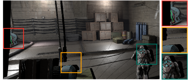
Fig. 2. An extrapolated frame by directly projecting fragments from the previously rendered frame. The right column shows three types of disocclusions: out-of-screen disocclusion , static disocclusion , and dynamic disocclusion from top to bottom. The thin black lines splatted in the image are due to forward warping.
