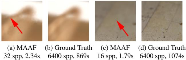
**Figure 13: Image insets from CONFERENCE (a)(b) and SPONZA (c)(d).** Our method produces results close to the ground truth generally. But there are some subtle artifacts: (a). Discontinuity around shadow and focal plane boundaries, where the double wedge shape changes a lot in nearby pixels. (c). Oversmoothed region.
