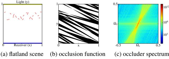
**Figure 4:** Numerical simulation of a flatland scene for soft shadows (a) Scene setup, similar to Fig. 7 in [EHDR11]. (b) Graph of occlusion function. (c) Fourier spectrum. Notice higher energy in the center of the double wedge, and falloff further from the origin.
