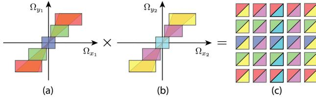
**Figure 7:** Constructing 4D MAAF filters from 2D filters along orthogonal dimensions, using different colors to distinguish different components. (a) 5 components in  $(\Omega_{x_1}, \Omega_{y_1})$ . (b) 5 components in  $(\Omega_{x_2}, \Omega_{y_2})$ . (c) When multiplied in the frequency domain to cover the 4D spectrum, these result in 25 filters in 4D.
