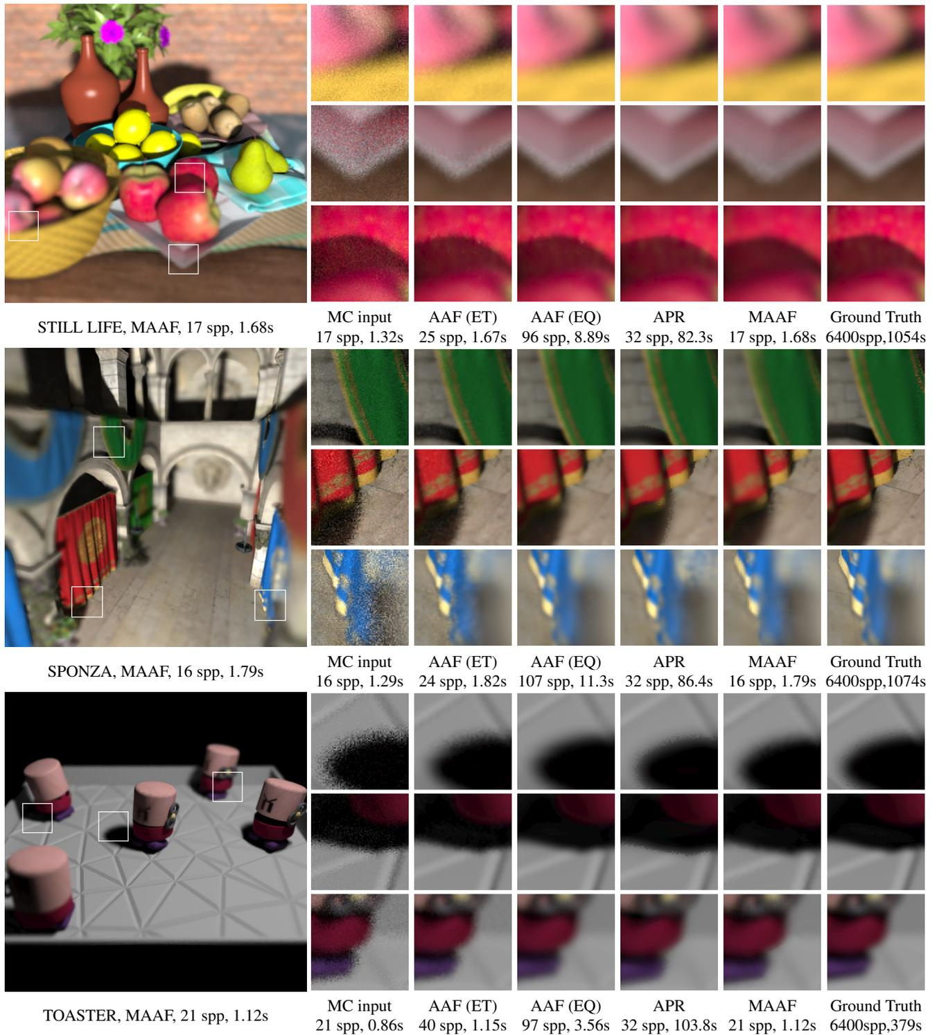
**Figure 14:** Scenes with multiple distribution effects together: defocus, soft shadows, and indirect illumination. We compare MAAF results to those obtained by AAF equal time and equal quality, as well as the state of the art offline denoising method, adaptive polynomial rendering (APR). MAAF usually obtains a speedup of about  $6\times$  with high quality results.
