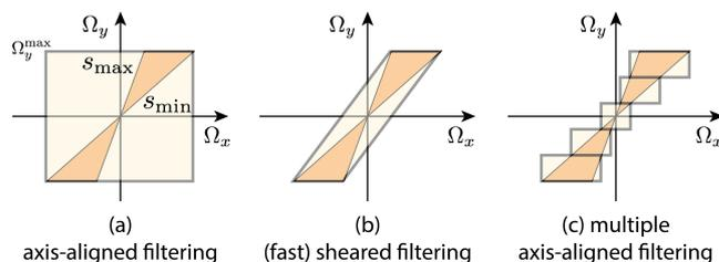
**Figure 1:** 2D filters for (a) axis-aligned filtering (AAF), (b) fast sheared filtering (FSF), and (c) our new multiple axis-aligned filtering (MAAF) with 5 filters. MAAF has the tightest fit (including in our practical implementation, which uses Gaussian filters), while enabling the simplicity and efficiency of single-pass axis-aligned filtering. In all cases, we seek to approximate the wedge Fourier spectrum bounded by slopes  $s_{\min}$  and  $s_{\max}$ , with bandwidth  $\Omega_y^{\max}$ .
