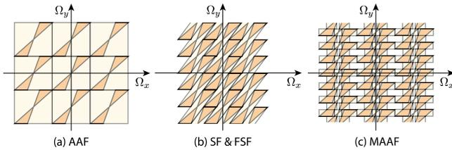
**Figure 3:** Showing replicas from sampling, and how large empty space in axis-aligned filtering leads to a higher sampling rate. Sheared filtering and our multiple axis-aligned filter method lead to much tighter packing of replicas, and lower sampling rates.
