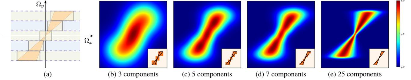
**Figure 5:** Progressively more compact and accurate approximations of the double wedge with more component filters in MAAF. Insets show a schematic with a number of box filters; we actually use weighted gaussians for the filters. (a) is a schematic with 5 filters typically used.
