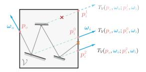
Fig. 14. To obtain reference samples for the appearance network, we can, in a single pass, aggregate multiple throughput samples for different exitant position  $\boldsymbol{p_i}$ . A red cross indicates a failed shadow test, while an orange cross indicates path termination at the voxel boundary.
