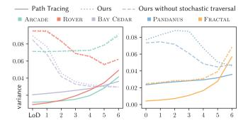
Fig. 17. Our approach does not apply any importance sampling and therefore has high per-pixel variance at higher detail levels. However, variance of our method is reduced as detail is reduced, while path tracing complexity stays constant due to tracing the same light paths. Our stochastic traversal incurs a minor addition of variance.
