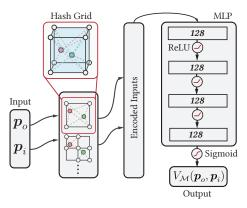
Fig. 7. Our visibility network architecture. Our recurrent composite encoding enables a single hash grid to be used by both inputs.
