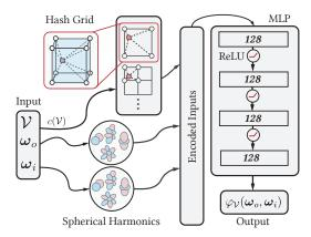
Fig. 5. Our appearance network architecture, where  $c(\mathcal{V})$  denotes the centre of the voxel  $\mathcal{V}$ .
