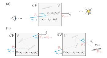
Fig. 3. Two configurations are possible in our generalised voxel path space. (a) If  $c_i = 0$  the subsequent interaction is entirely defined by a single direction. (b) If  $c_j = 1$ , an additional positional offset  $p'_i$  of pre-scattering incidence is tracked. Subsequent vertex positions  $p_{i+1}$  fall either onto the next voxel boundary or onto any non-voxelised geometry in  $(\mathcal{M} \setminus \mathcal{M}_{\overline{\mathcal{M}}})$ .
