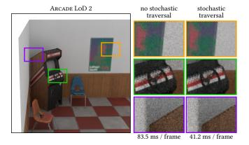
Fig. 11. Our stochastic traversal trades variance for efficiency. We compare to our approach without stochastic traversal at LoD 2. Each method is rendered for 10 seconds at a higher pixel resolution to better show the noise difference. Our approach consistently achieves lower variance in the same time budget.
