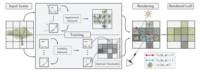
Fig. 4. Our neural asset prefiltering pipeline consists of a preprocessing part running local ray and path sampling on input assets to train our neural LoD representations for visibility and appearance, and a runtime evaluation part integrated with rendering.
