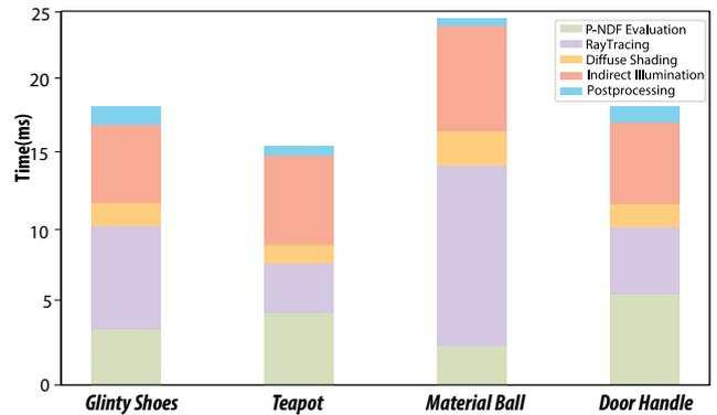
**Figure 15:** Computation time for each component (P-NDF evaluation, Ray tracing, Diffuse shading, Indirect illumination and Post-processing) in our algorithm for four scenes.
