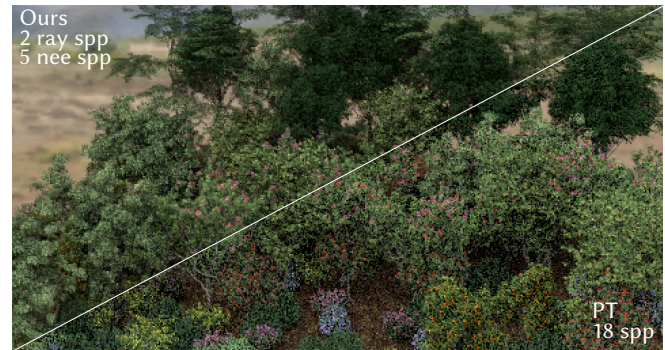
Fig. 17. Equal-time rendering comparison. Both images are rendered for 1 second. Our method performs splitting to improve efficiency by allocating 5 NEE samples per ray sample.
