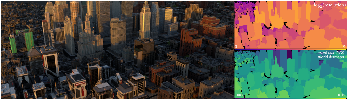
Fig. 1. Left: Metropolis , a cityscape rendered with our scene aggregation approach. The scene includes 82 unique buildings and 270 instances and originally requires 46.9 GB to store, making it challenging to render while stay in in-core memory. Our representation drastically reduces the size to 5.33 GB while preserving the detailed appearance. Right Top: Each instance selects the appropriate LoD resolution where the projected voxel size matches the pixel footprint (rounded to the nearest power of two). Right Bottom: As a result, close-view instances are rendered with finer voxels while distant instances are rendered with coarser voxels.
