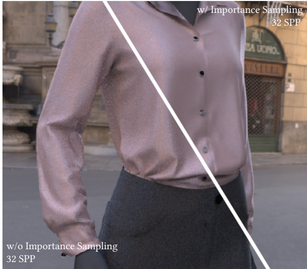
Figure 5: Importance sampling produces almost noise-free rendering with only 32 SPP under environment lighting. Both parts use our multi-scale model.
