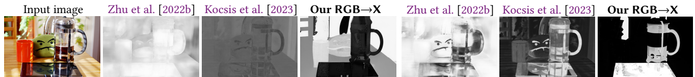
(c) Our RGB→X roughness estimation on the IIW dataset outperforms previous methods.
