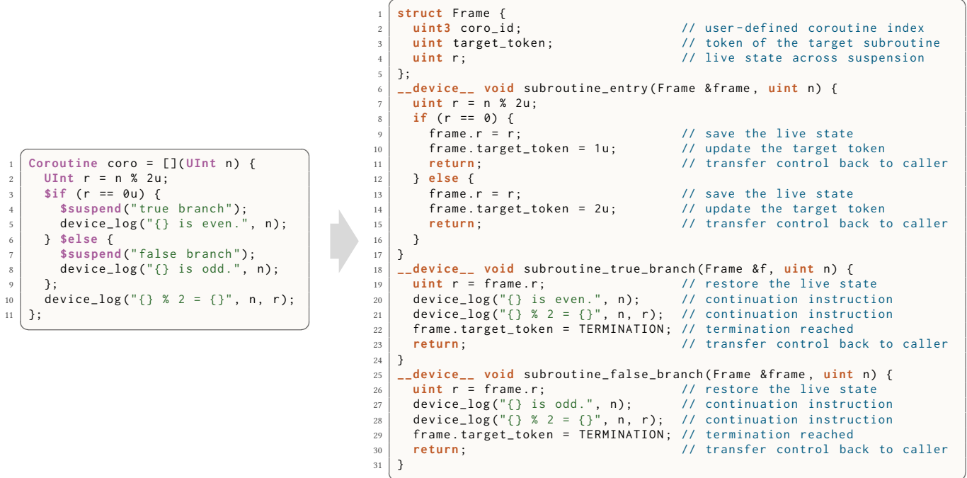
Fig. 5. An illustration of the internal representation of the state frame and extracted subroutines of a transformed Coroutine after compilation passes. Each subroutine is an ordinary LUISA Callable , where the first argument is the state frame and the remaining arguments are inherited from the original definition. Upon resumption, the subroutine reads the live states from the frame and executes the continuation instructions. When the next suspension point or termination is reached, the subroutine saves the live states and updates the target_token field of the frame.
