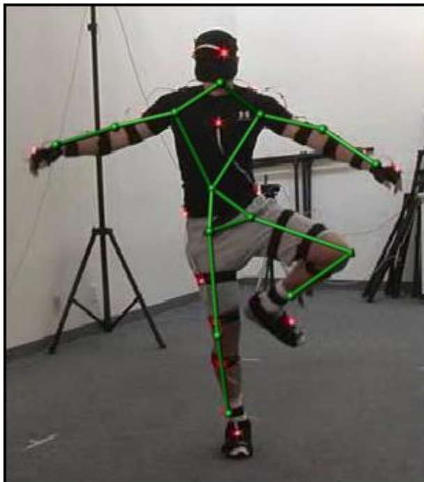
FIG. 10.5. An optical motion capture system in use (Kirk et al. 2005) (Copyright 2005 Adam Kirk, James O'Brien, and David Forsyth. Used with permission.)
