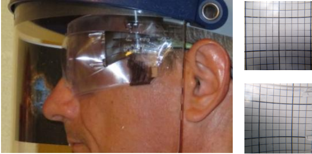
Figure 3: Left: Fresnel glasses with a head-mounted image plane (left eye image removed for clarity). Right: Views to front and 65° to the side.
