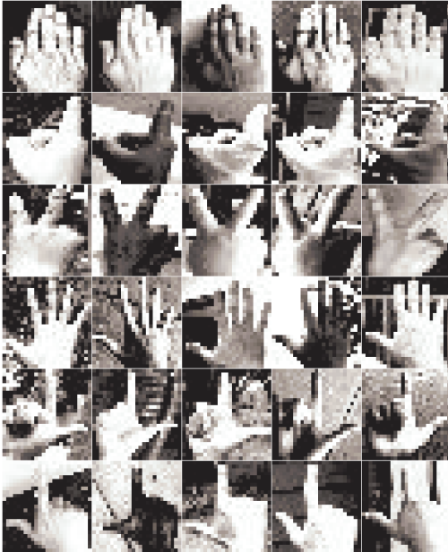
Figure 3: Sample areas of the six hand postures, from top to bottom: closed , sidepoint , victory , open , Lpalm , and Lback . They are shown in the smallest resolution necessary for detection (25x25).
