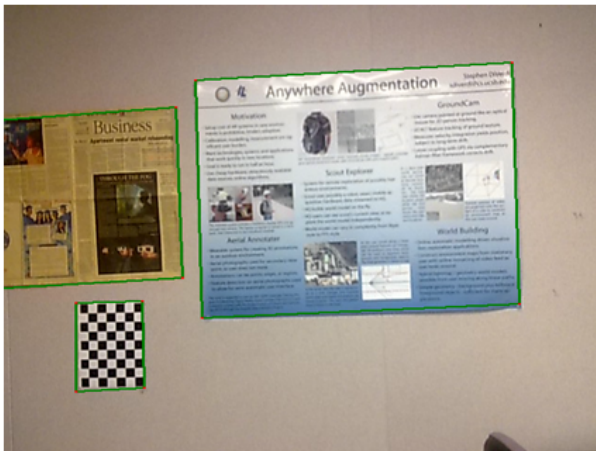
Figure 6. Augmented picture when the rotation between the database and the cell phone images is low. Accuracy is better.
