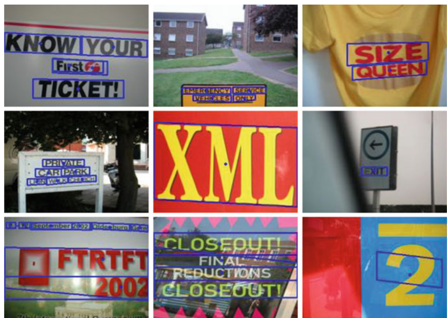
Fig. 1.4 Examples of good ( top and mid rows ) and bad ( bottom row ) text localization on the ICDAR 2003 dataset. The blue point in each quadrilateral represents the (simulated) input of the user. TranslatAR’s algorithm was able to very accurately detect the text at different scales and under perspective distortion. The failure cases are mostly due to very nonuniform background and/or lighting effects (first two). For very large letters, the expansion algorithm used to detect the texts bounding box can stop inside one of the letters ( bottom right )
