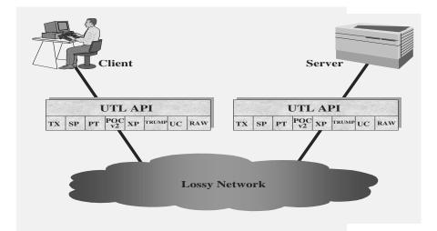
Fig. 3. How UTL is Used in Client/Server Applications
