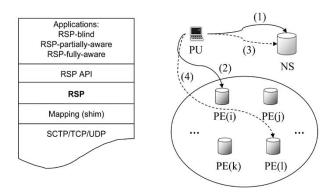
Fig. 1. Reliable server pooling: protocol stack and basic operations.
