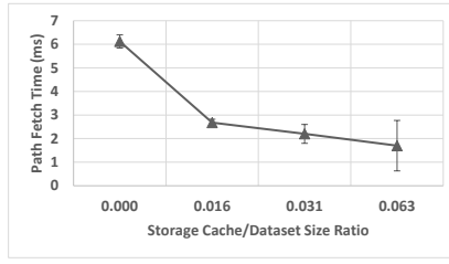
(b) Effect of caching at the untrusted server on average path fetch time from disk
