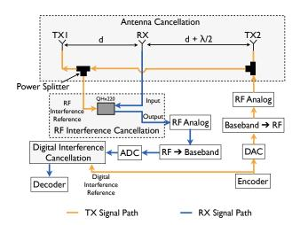
Figure 2: Block diagram of a wireless full-duplex node. Colored blocks correspond to different techniques for self-interference cancellation. The power splitters introduce a 6dB reduction in signal, thus power from TX1 is 6dB lower compared to power from TX2, without the need for an additional attenuator.
