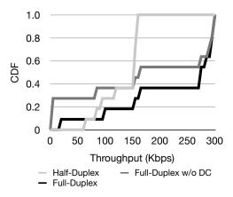
Figure 9: Aggregate throughput of half-duplex links, full-duplex without digital interference cancellation, and full-duplex. Full-duplex links can achieve 84% higher median throughput.
