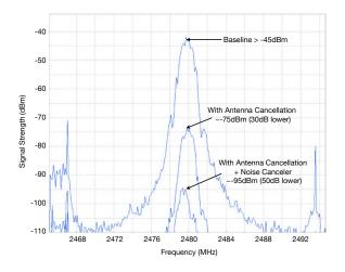
Figure 7: Spectrum snapshots showing the effect of antenna cancellation and a combination of antenna and RF interference cancellation. A combination of the two techniques can give a  $\sim$ 50dB reduction in self-interference.
