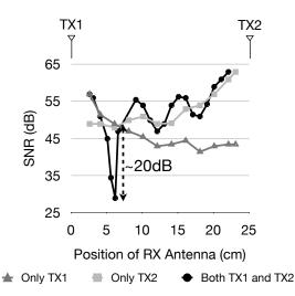
Figure 5: Received SNR for different receive antenna placements. The received SNR is fairly monotonic with distance when any one transmit antenna is active. With both transmit antennas active, there is a sharp reduction in receive power at the null point.
