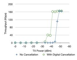
Figure 1: Receive throughput at a node with selfinterference using digital interference cancellation. Digital interference cancellation gives an SNR gain of only about 10dB.
