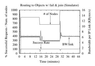
Fig. 20. Route to Object under failure and joins. The performance of Tapestry route to objects with two massive network membership change events. Starting with 830 nodes, 20% of nodes (166) fail, followed 16 minutes later by a massive join of 50% (333 nodes).
