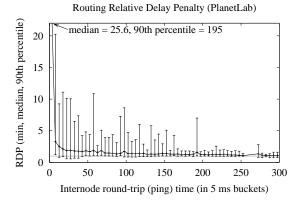
Fig. 13. *RDP of Routing to Nodes*. The ratio of Tapestry routing to a node versus the shortest roundtrip IP distance between the sender and receiver.
