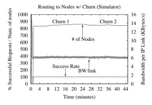
Fig. 21. Route to Node under churn. Routing to nodes under two churn periods, starting with 830 nodes. Churn 1 uses a poisson process with average inter-arrival time of 20 seconds and randomly kills nodes such that the average lifetime is 4 minutes. Churn 2 uses 10 seconds and 2 minutes.
