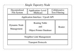
Fig. 6. Tapestry component architecture. Messages pass up from physical network layers and down from application layers. The Router is a central conduit for communication.
