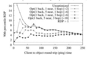
Fig. 15. 90<sup>th</sup> percentile RDP of Routing to Objects with Optimization. Each line represents a set of optimization parameters (*k* backups, *l* nearest neighbors, *m* hops), with cost (additional pointers per object) in brackets.
