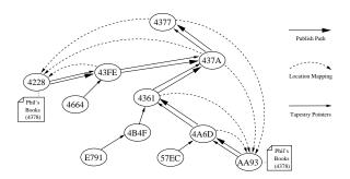
Fig. 4. Tapestry object publish example. Two copies of an object (4378) are published to their root node at 4377. Publish messages route to root, depositing a location pointer for the object at each hop encountered along the way.
