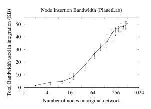
Fig. 17. Node Insertion Bandwidth. Total control traffic bandwidth for single node insertion.
