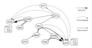
Fig. 5. *Tapestry route to object example.* Several nodes send messages to object 4378 from different points in the network. The messages route towards the root node of 4378. When they intersect the publish path, they follow the location pointer to the nearest copy of the object.
