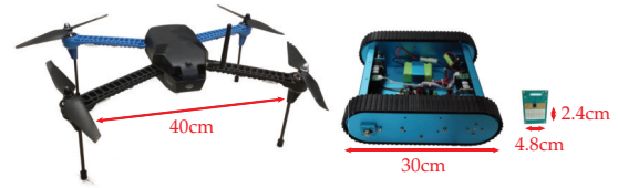
Figure 3: The actual size comparison of a drone, a robot car and our 60GHz array prototype. The array (16×8) is compact and both TX and RX can be mounted on a single mobile device.
