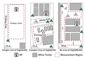
Figure 3: Graphical illustration of the three propagation environments used in our experiments, all located on the UC Santa Barbara campus. For both Complex LOS and NLOS, the AP was mounted right below the roof of an office trailer, and there are many static and moving obstacles nearby, including trees, cars, bikers and pedestrians. For NLOS, the path between the AP and the measured region is blocked by office trailers.
