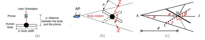
Figure 4: An abstract model of the human shield effect. (a) A simple model of a user holding a smartphone, with body width b and phone/body distance p. (b) The signal propagation condition as the user rotates. When the user orientation is between  $\vec{d_1}$  and  $\vec{d_2}$ , the LOS path will be blocked by the human body. This range of orientation is referred to as the blocking sector. (c) A geometric representation of the blocking sector.
