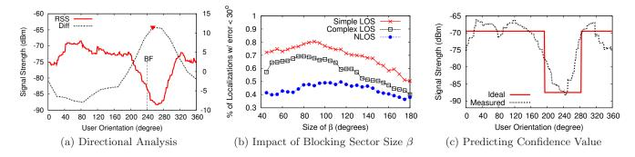
Figure 5: Borealis' directional analysis. (a) Deriving the AP direction based on the blocking sector.(b) Choosing the blocking sector size. (c) Predicting the confidence of our direction analysis by computing the cross-correlation between the measured and ideal signal strength profiles.
