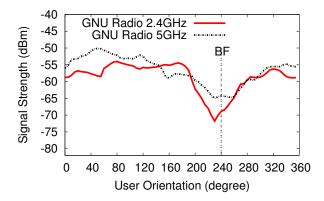
Figure 11: Sample signal strength profiles as a user rotates, measured using USRP2 GNU radios operating on 2.4GHz and 5GHz. We observe the same signal-blocking artifact. As before, BF marks the direction where the user has her back facing the AP.
