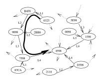
Figure 1: *Routing example in a structured overlay using prefix routing*. Node 5230 routes a message to the key 8954. At each hop the message is forwarded to a node that shares a longer prefix with the key.
