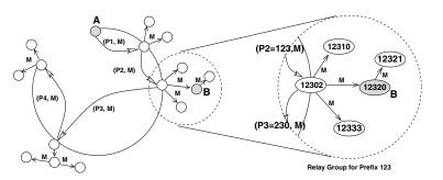
Figure 2: A forwarding path from A to B composed of multiple relay groups. Here a relay group is defined by a 3-digit prefix. At each relay group, the first node to receive the message broadcasts the message to all members of the group using *directed broadcast*. In the inset, node 12302 forwards the message to the rest of the relay group for prefix 123.
