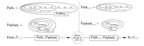
Figure 3: A detailed look at the path and payload components of a message, before and after processing at a relay group. The relay group root for  $P_i$  decrypts the layer around the path component to get  $P_{i+1}$ ,  $R_i$ ,  $K_i$ . It performs a symmetric decryption on the payload using  $R_i$ , and forwards the result to the relay group  $P_{i+1}$ .
