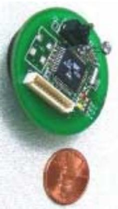
**Figure 8: A TinyOS-based Mote:** This “mote” includes a 4MHz microcontroller, a software-driven radio, and an application that coordinates with neighboring motes to discover an ad-hoc sensor network routing topology.
