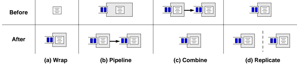
Figure 3: **The Four Design Patterns:** The four design patterns, **wrap**, **pipeline**, **combine**, and **replicate**, can be applied to stages of a service to condition it against load, failures, and limited or bottleneck resources.
