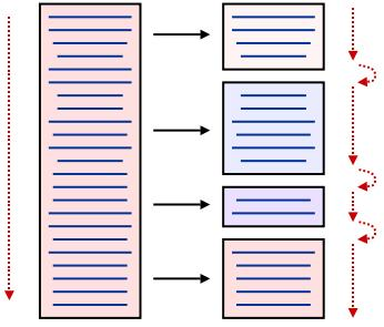
Figure 2: **Splitting a Service into Stages:** Our programming model views a service as a sequence of stages, separated by high- or variable-latency operations. Stages only share data using pass-by-value semantics, for example, by exchanging messages.
