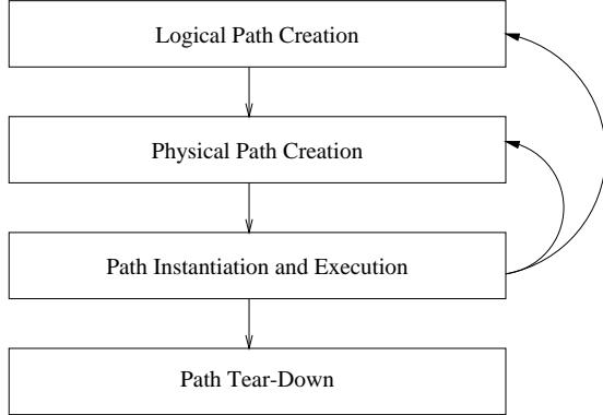
**Figure 11: Path construction process:** Path execution is an iterative process of optimization. The Ninja APC facility guarantees the availability and fault-tolerance of a constructed path by rebuilding its physical or logical path.
