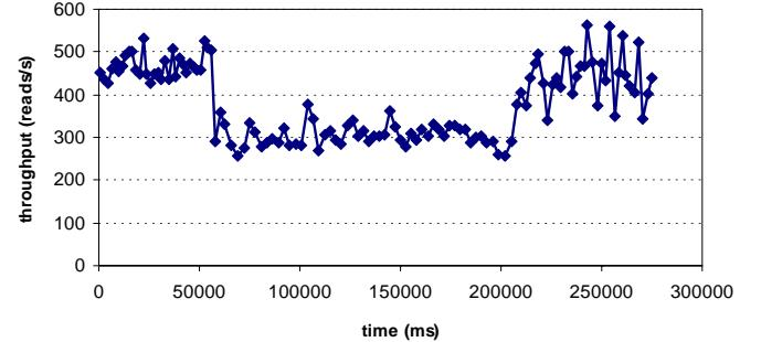
Figure 7: **Availability and Recovery:** This benchmark shows the read throughput of a 3 node hash table as a deliberate single-node fault is induced, and afterwards as recovery is performed.
