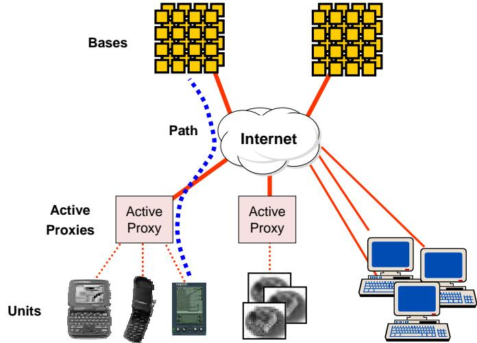
**Figure 1: The Ninja Platform Architecture:** The architecture consists of bases (services running on clusters of workstations), active proxies (stateless or soft-state intermediaries between units and services), units (heterogeneous devices and sensors), and paths (a composition chain across units, proxies, and services in bases).
