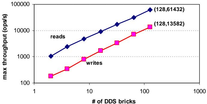
Figure 6: **Throughput scalability:** This benchmark shows the linear scaling of throughput as a function of the number of bricks serving in a distributed hash table; note that both axis have logarithmic scales. As we added more bricks to the DDS, we increased the number of workers using the DDS until throughput saturated.
