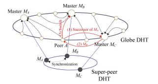
Fig. 9. The cluster-based architecture. Peers are organized into storage clusters, each of which has a master peer (locatable by searching for the master ID in the globe DHT) which monitors and maintains replicas of objects stored in the cluster, and resolves client queries.
