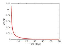
Fig. 7. Complementary cumulative distribution of failure-recovery times.
