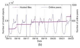
Fig. 11. The evolution of the remaining replicas over a week period (September 15-22, 2009). (a) Average number of remaining replicas per object. (b) Number of objects and online peers along with time (the ticks on the x-axis correspond to midnight (00:00 am) on the days that are labeled).
