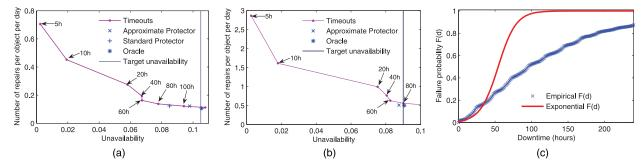
Fig. 8. Performance of Protector with the real trace-driven simulation in the Maze environment. (a) Cost-availability trade-off under replication scheme ( $t_r = 7$ ). (b) Cost-availability trade-off under coding scheme (b = 6,  $t_r = 32$ ). (c) Comparison between empirical F(d) and exponential F(d).
