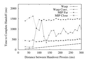
Figure 9: *Handoff latency* as a function of density of adjacent proxies or base stations. For Mobile IP, we measure both when the MN is close and far from home. Warp converge is the time to full routing state convergence.
