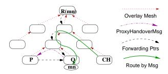
Figure 4: *Updating a location binding via ProxyHandoverMsg.* Correspondent host CH sends a message to mobile node mn after mn moves from proxy P to Q.
