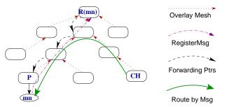
Figure 3: *Communicating with a mobile host.* Mobile node mn registers with proxy P, and correspondent host CH sends a message to mn.
