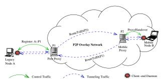
Figure 5: *Tunneling legacy application traffic through client-end daemons and overlay proxies.* A legacy node A communicates with mobile node B.
