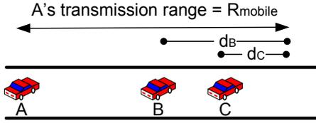
Fig. 3. Position-guided group broadcast. When vehicles  $B$  and  $C$  receive  $A$ 's broadcast of data  $i$ , both initiate a local timer that is proportional to their distance to the edge of  $A$ 's transmission range,  $d_B$  and  $d_C$ .
