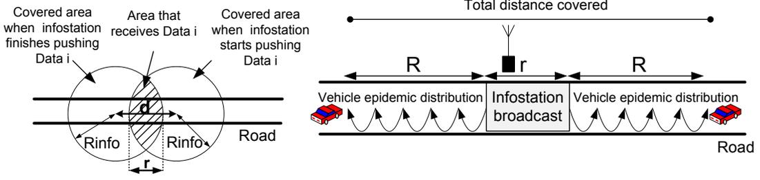
Fig. 1. Coverage of push. (Left) Coverage of infostation's broadcast. Nodes which obtain the complete content of data  $i$  are only in the shaded area.  $d = \frac{S}{B_{info}}V$ . If  $d \geq 2R_{info}$  then the shaded area is NULL, i.e. no node can download the complete set of data  $i$ . (Right) Coverage of subsequent vehicle epidemic content distribution. Vehicles propagate data  $i$  to both directions in multi-hops.
