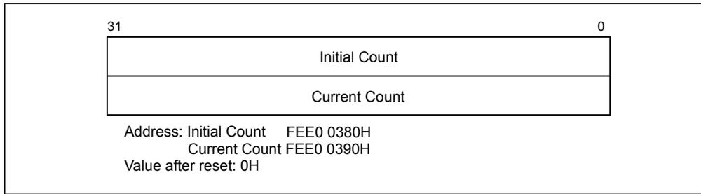
**Figure 10-11. Initial Count and Current Count Registers**
