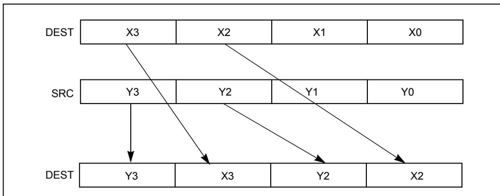
Figure 4-24. UNPCKHPS Instruction High Unpack and Interleave Operation
