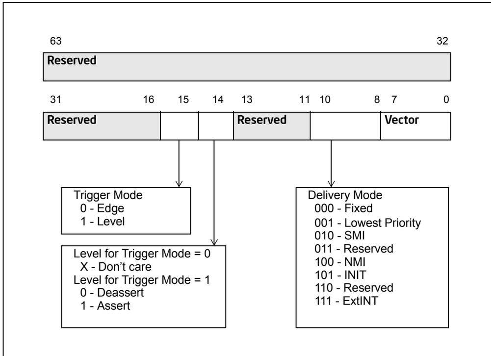
Figure 10-25. Layout of the MSI Message Data Register
