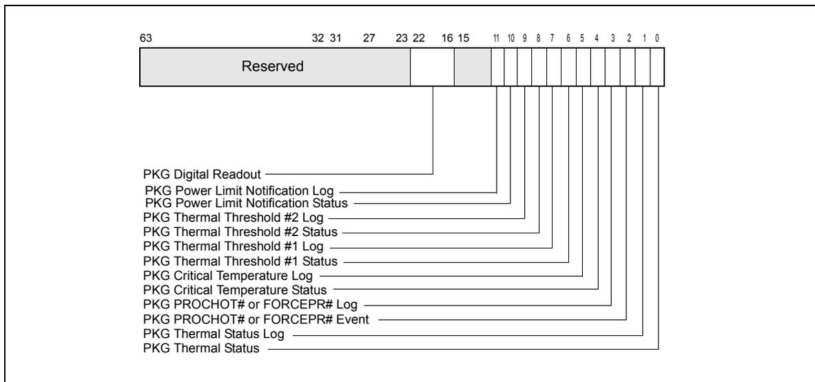
Figure 14-30. IA32\_PACKAGE\_THERM\_STATUS Register
