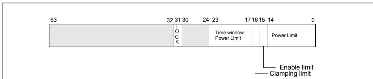
Figure 14-37. MSR\_PP0\_POWER\_LIMIT/MSR\_PP1\_POWER\_LIMIT Register
