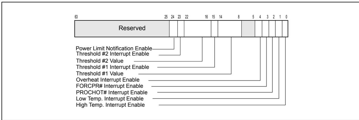
Figure 14-29. IA32\_THERM\_INTERRUPT Register
