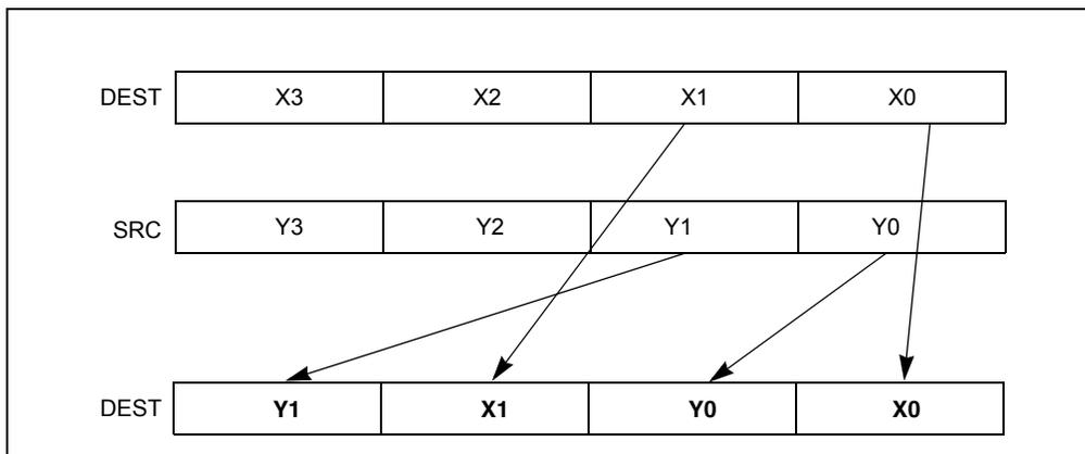
Figure 4-26. UNPCKLPS Instruction Low Unpack and Interleave Operation
