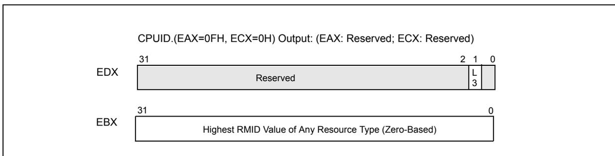
Figure 17-20. CPUID.(EAX=0FH, ECX=0H) QoS Monitoring Resource Type Enumeration
