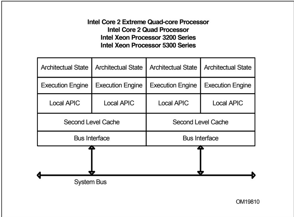
**Figure 2-7. Intel 64 Processors that Support Quad-Core**
