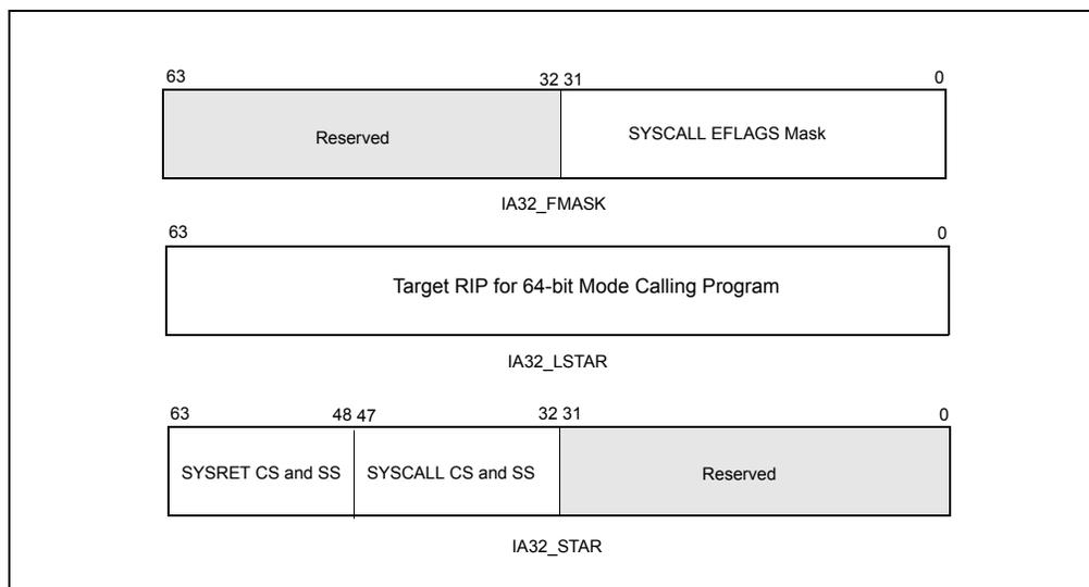
**Figure 5-14. MSRs Used by SYSCALL and SYSRET**
