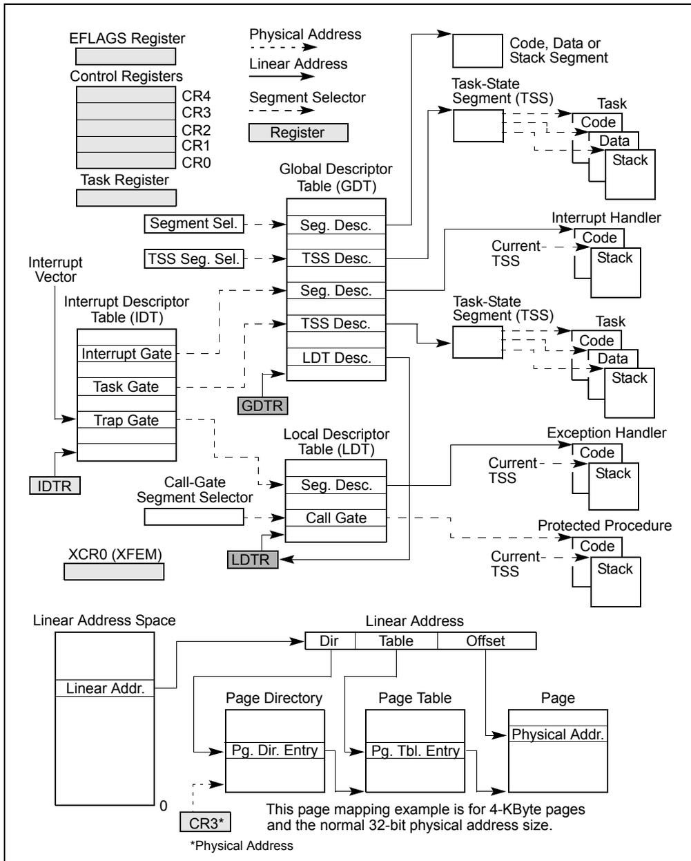
Figure 2-1. IA-32 System-Level Registers and Data Structures
