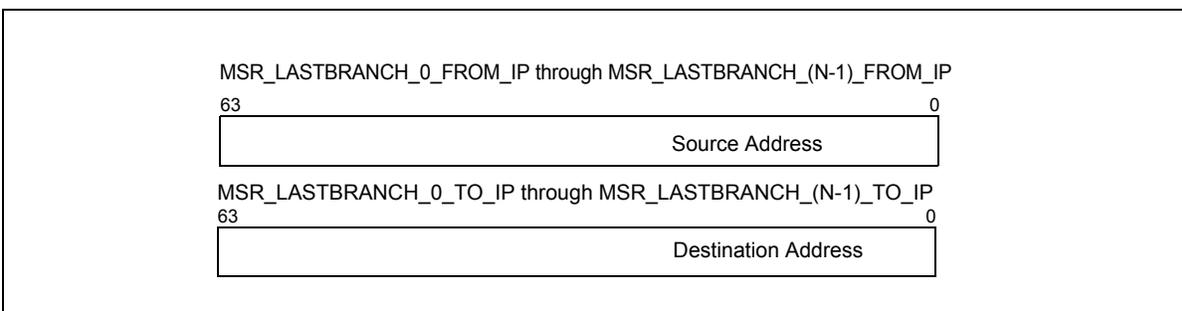
Figure 17-4. 64-bit Address Layout of LBR MSR
