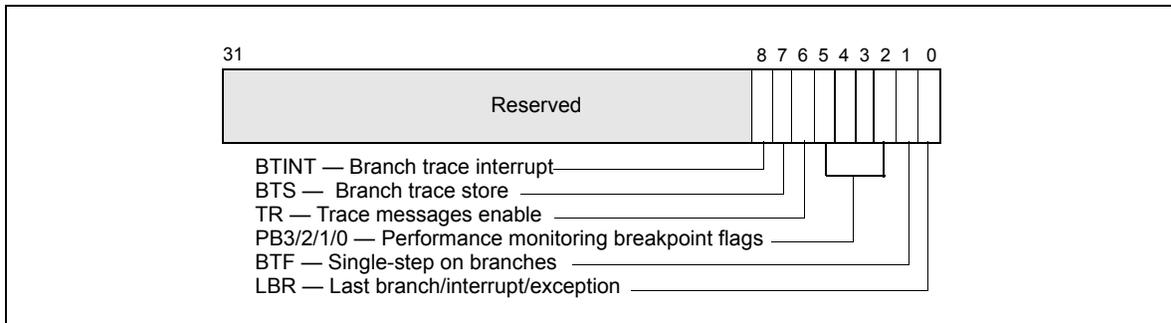
Figure 17-16. MSR\_DEBUGCTLB MSR for Pentium M Processors
