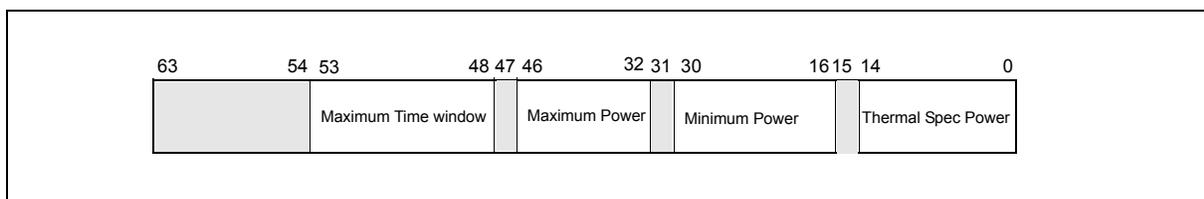
Figure 14-35. MSR\_PKG\_POWER\_INFO Register
