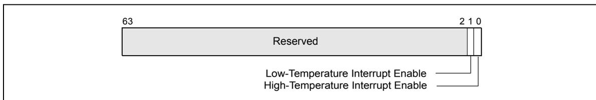
Figure 14-25. IA32\_THERM\_INTERRUPT MSR
