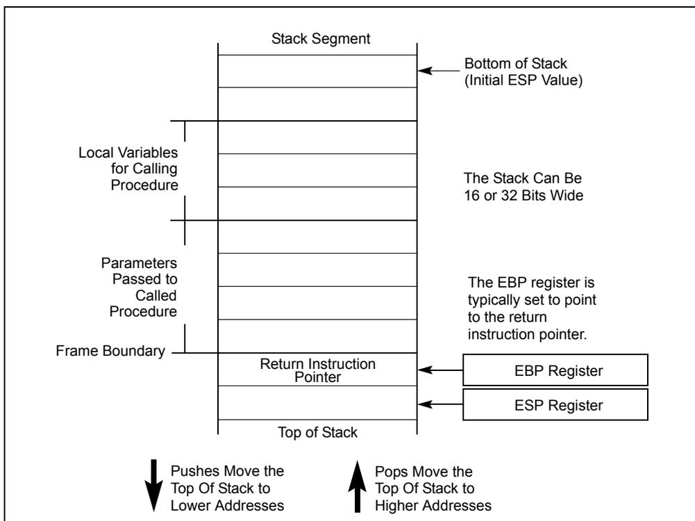
Figure 6-1. Stack Structure
