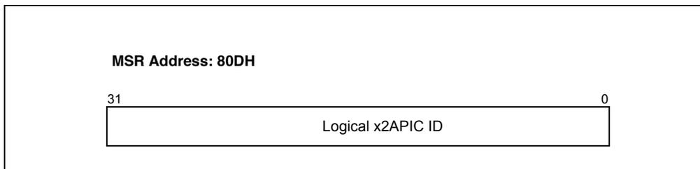
**Figure 10-29. Logical Destination Register in x2APIC Mode**
