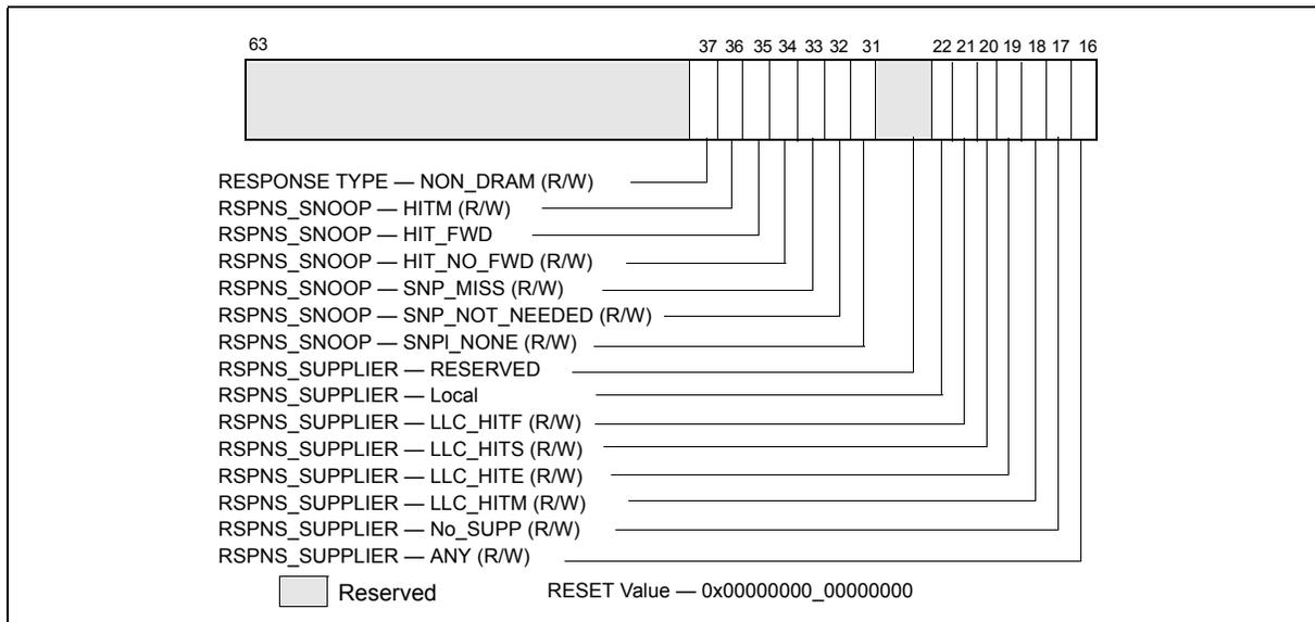
**Figure 18-33. Response\_Supplier and Snoop Info Fields for MSR\_OFFCORE\_RSP\_x**
