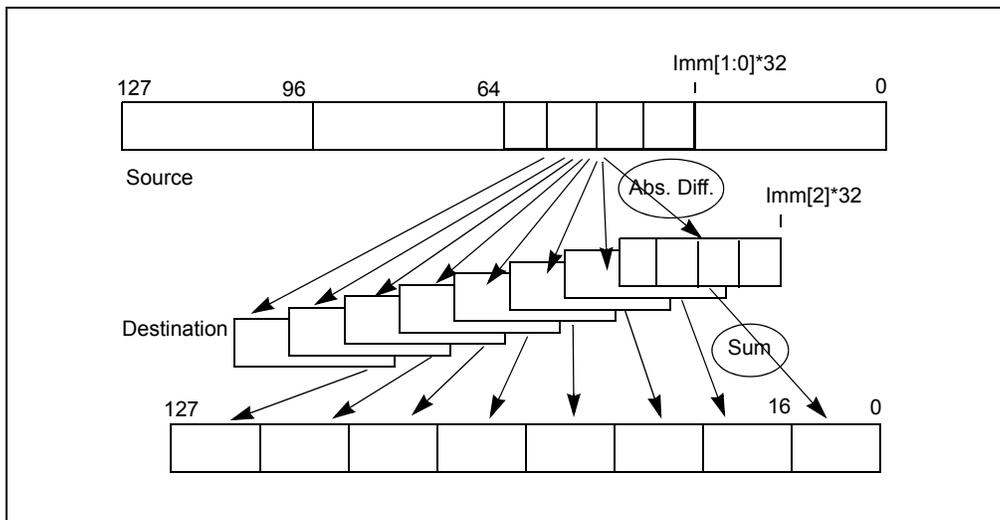
**Figure 12-4. MPSADBW Operation**
