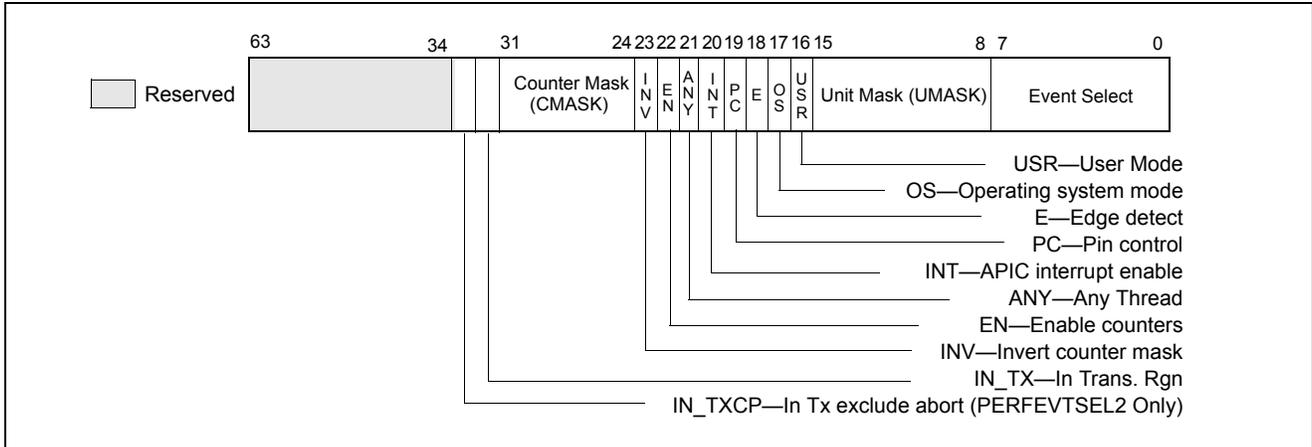
**Figure 18-36. Layout of IA32\_PERFEVTSELx MSRs Supporting Intel TSX**
