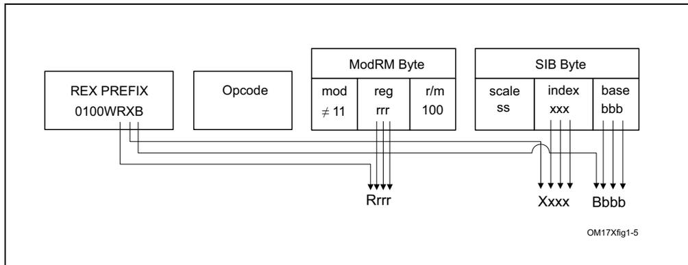
**Figure 2-6. Memory Addressing With a SIB Byte**
