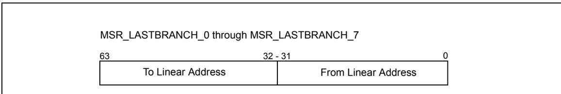
Figure 17-15. LBR Branch Record Layout for the Intel Core Solo and Intel Core Duo Processor
