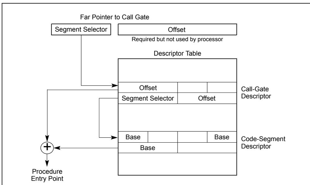
Figure 5-10. Call-Gate Mechanism
