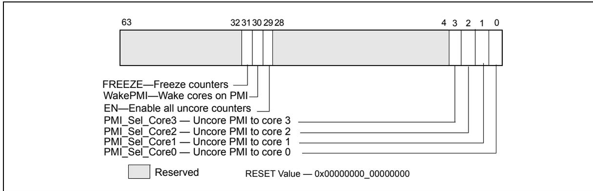
Figure 18-35. Layout of MSR\_UNC\_PERF\_GLOBAL\_CTRL MSR for Uncore
