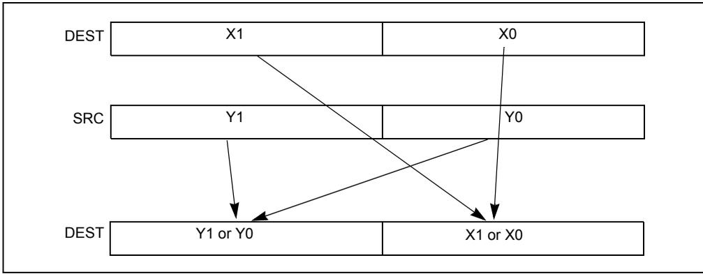
**Figure 11-5. SHUFPD Instruction, Packed Shuffle Operation**
