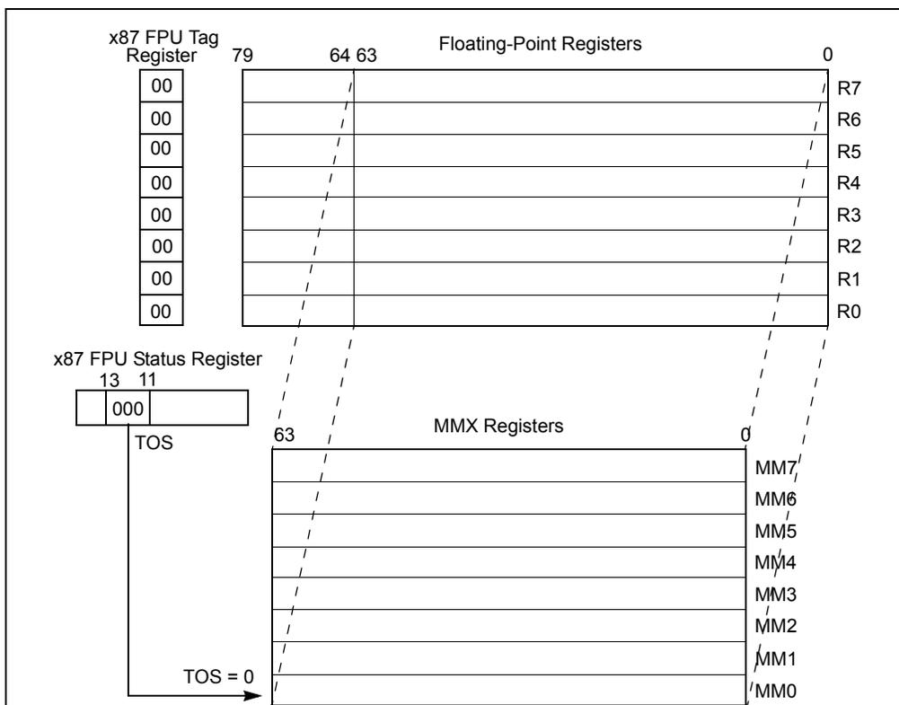
**Figure 12-1. Mapping of MMX Registers to Floating-Point Registers**
