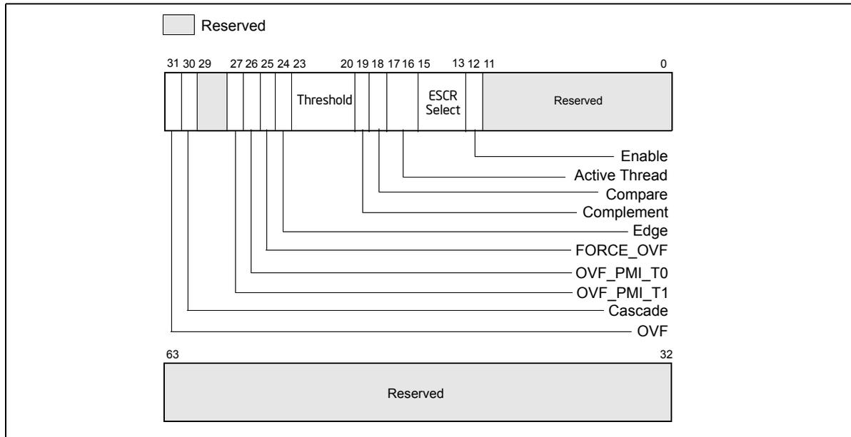
**Figure 18-42. Counter Configuration Control Register (CCCR)**
