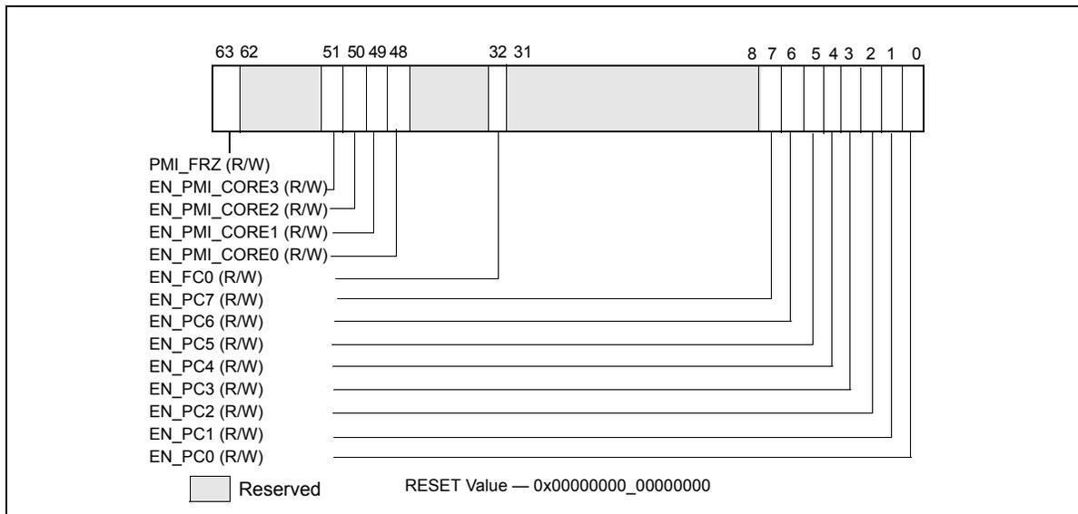
Figure 18-21. Layout of MSR\_UNCORE\_PERF\_GLOBAL\_CTRL MSR
