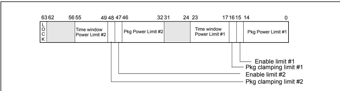
**Figure 14-33. MSR\_PKG\_POWER\_LIMIT Register**
