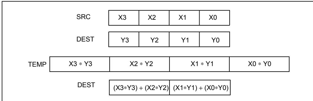
Figure 4-7. PMADDWD Execution Model Using 64-bit Operands
