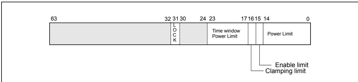
Figure 14-41. MSR\_DRAM\_POWER\_LIMIT Register
