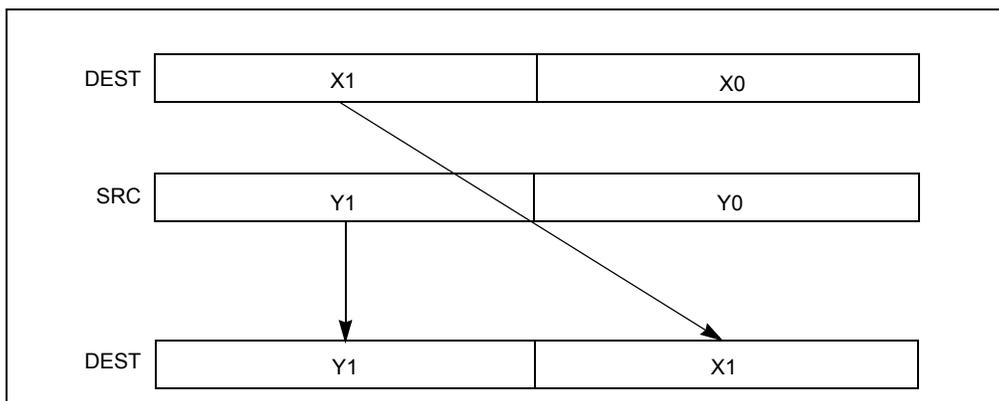
Figure 4-23. UNPCKHPD Instruction High Unpack and Interleave Operation
