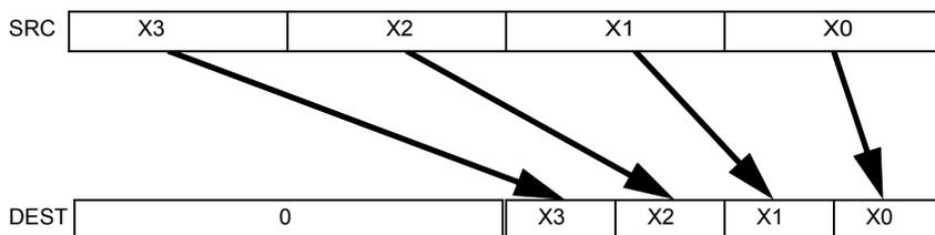
Figure 3-12. VCVTPD2PS (VEX.256 encoded version)
