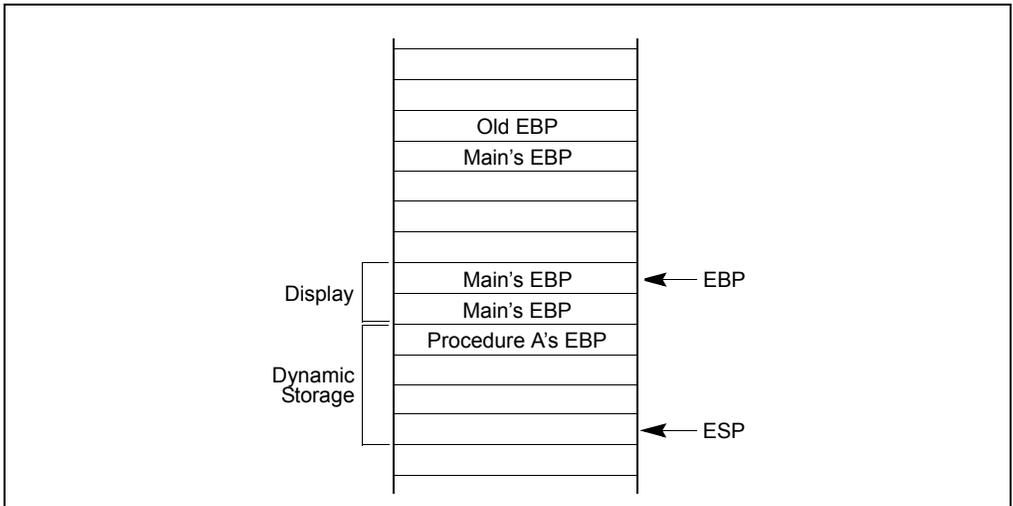
Figure 6-8. Stack Frame After Entering Procedure A
