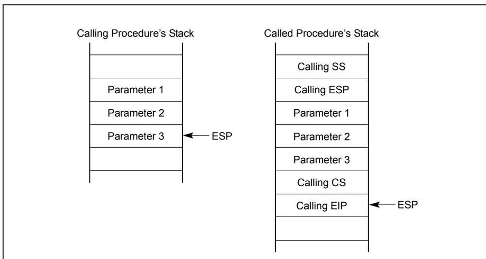
**Figure 5-13. Stack Switching During an Interprivilege-Level Call**
