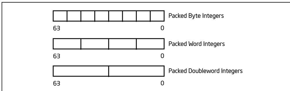
**Figure 9-3. Data Types Introduced with the MMX Technology**
