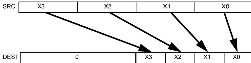
Figure 3-14. VCVTTPD2DQ (VEX.256 encoded version)
