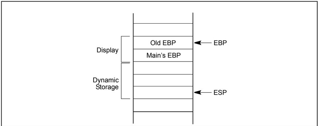
Figure 6-7. Stack Frame After Entering the MAIN Procedure
