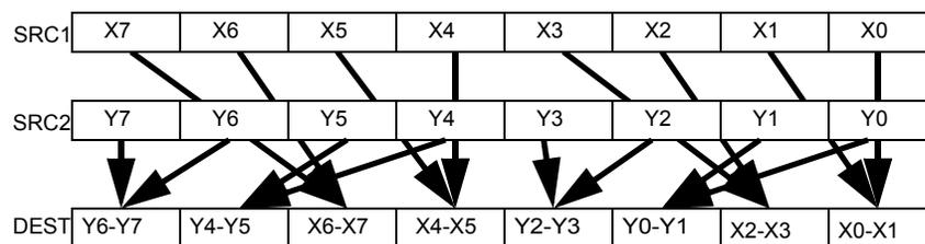
**Figure 3-22. VHSUBPS operation**
