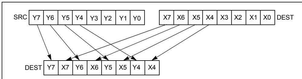
Figure 4-16. PUNPCKHBW Instruction Operation Using 64-bit Operands
