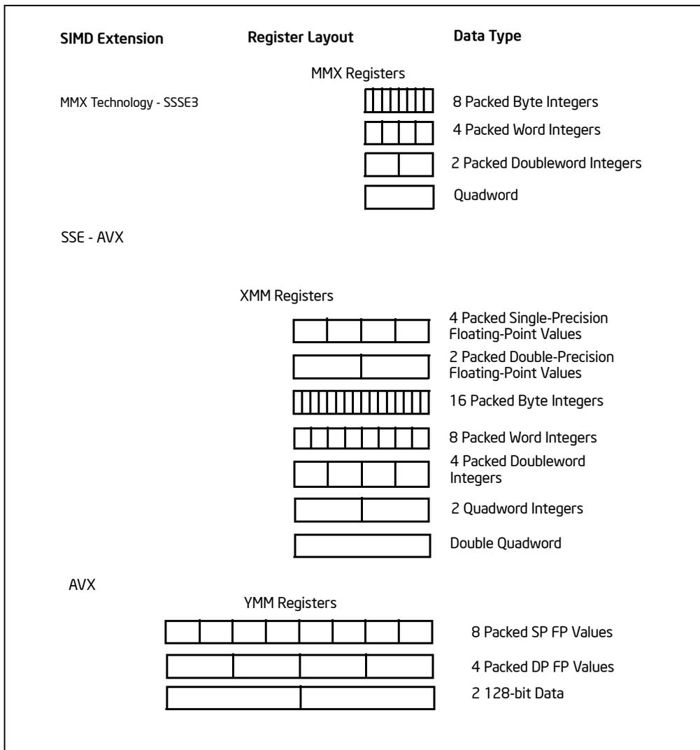
Figure 2-4. SIMD Extensions, Register Layouts, and Data Types
