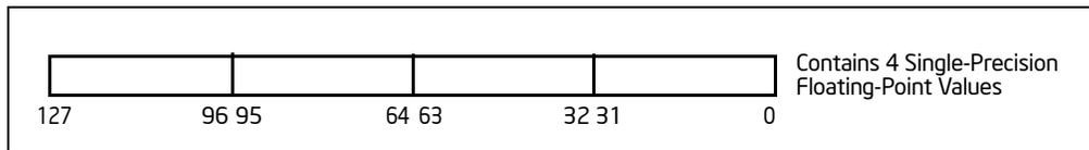
**Figure 10-4. 128-Bit Packed Single-Precision Floating-Point Data Type**
