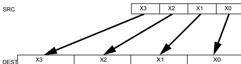
Figure 3-13. CVTPS2PD (VEX.256 encoded version)
