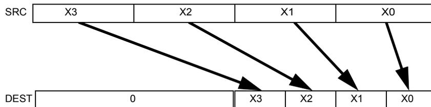
Figure 3-11. VCVTPD2DQ (VEX.256 encoded version)
