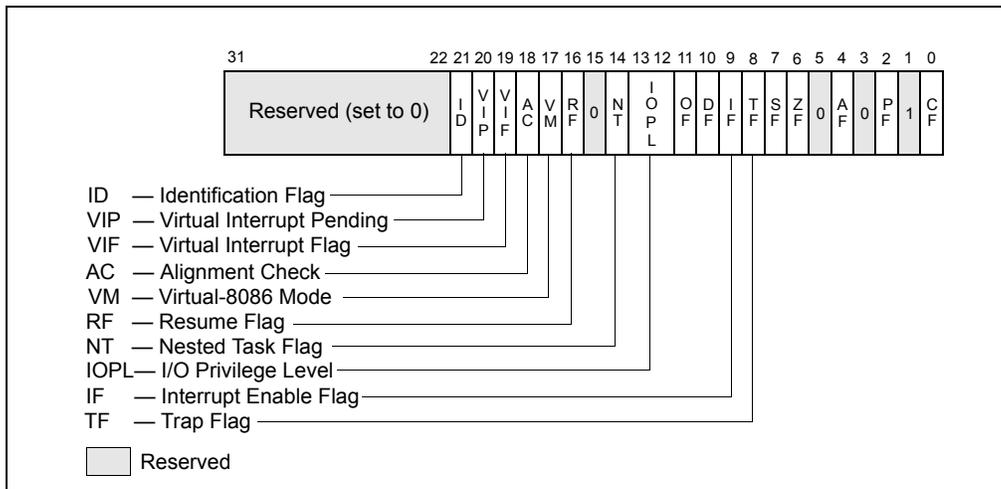
Figure 2-5. System Flags in the EFLAGS Register
