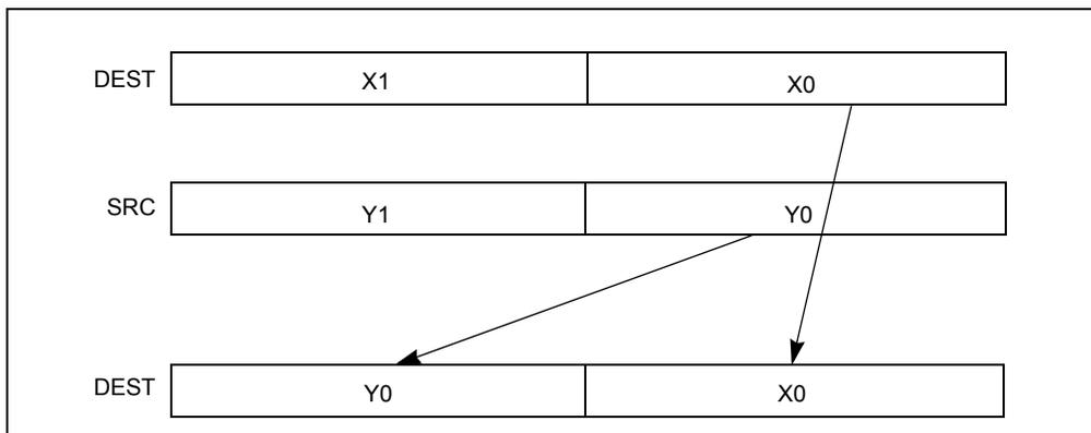
Figure 4-25. UNPCKLPD Instruction Low Unpack and Interleave Operation
