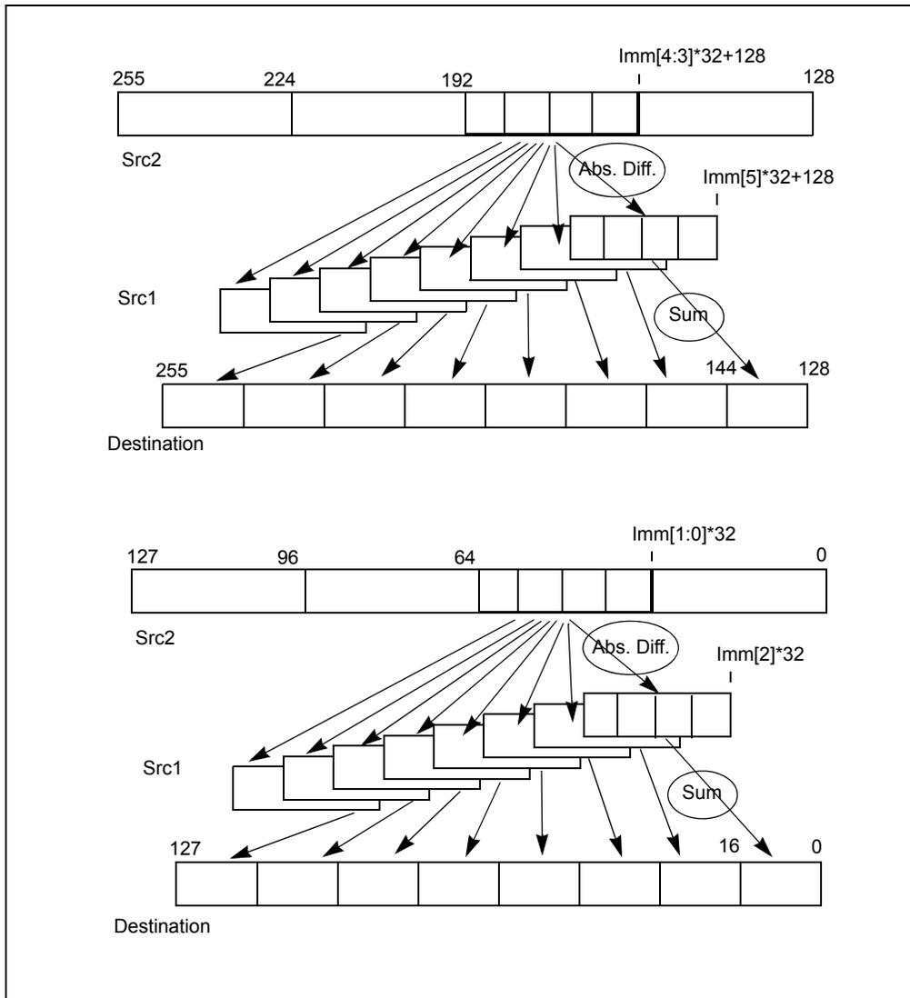
Figure 3-27. VMPSADBW Operation
