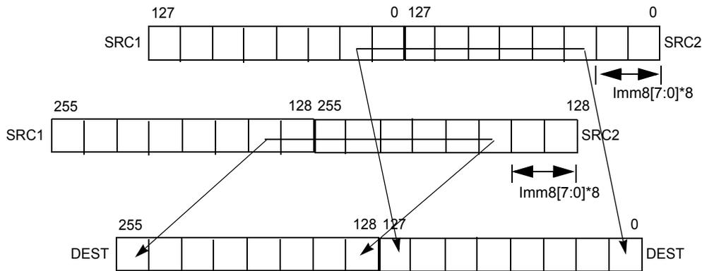
Figure 4-3. 256-bit VPALIGN Instruction Operation
