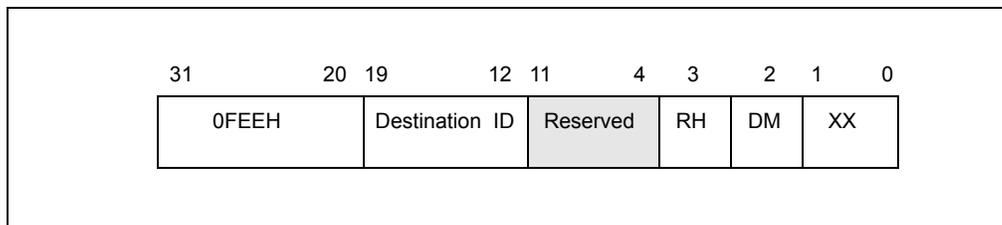
Figure 10-24. Layout of the MSI Message Address Register
