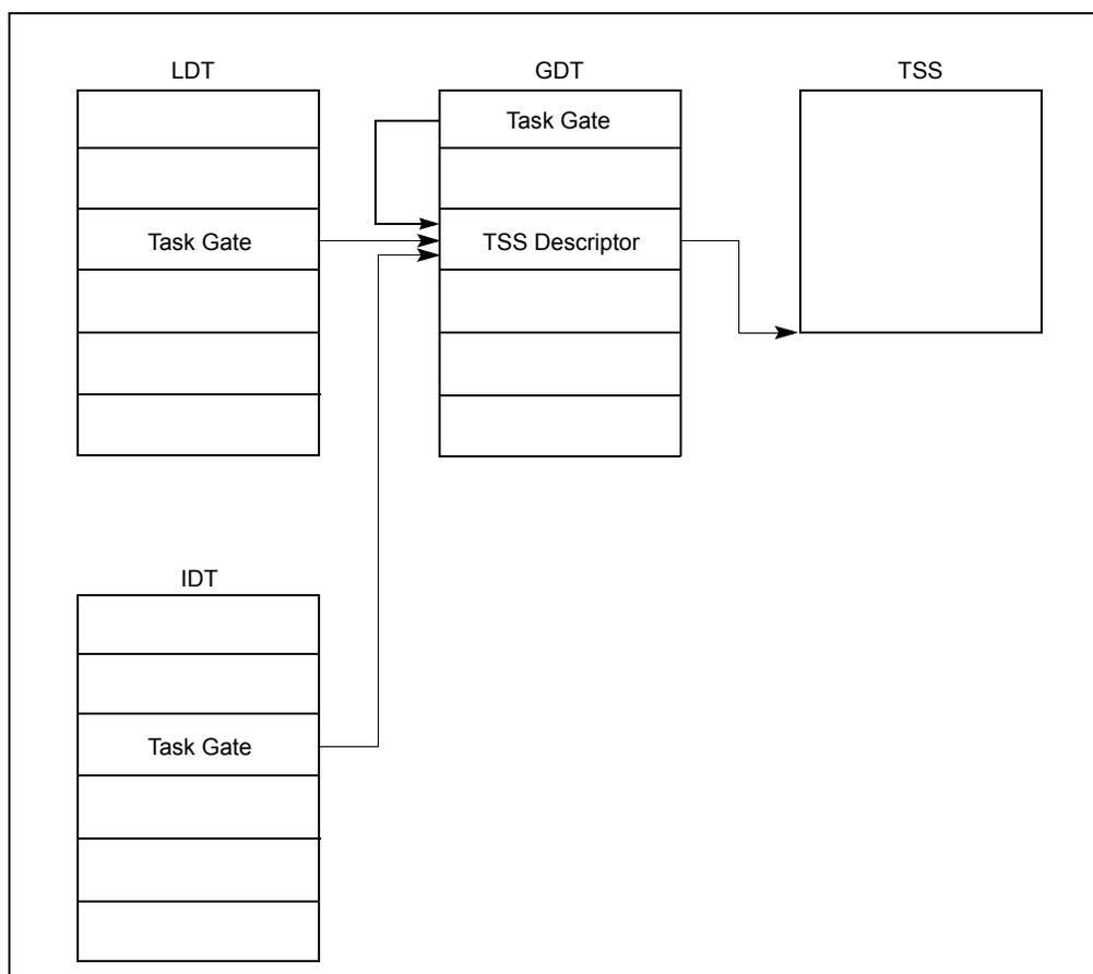
Figure 7-7. Task Gates Referencing the Same Task
