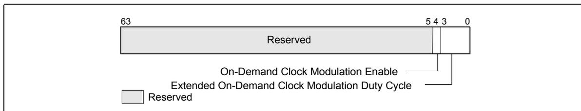
**Figure 14-27. IA32\_CLOCK\_MODULATION MSR with Clock Modulation Extension**
