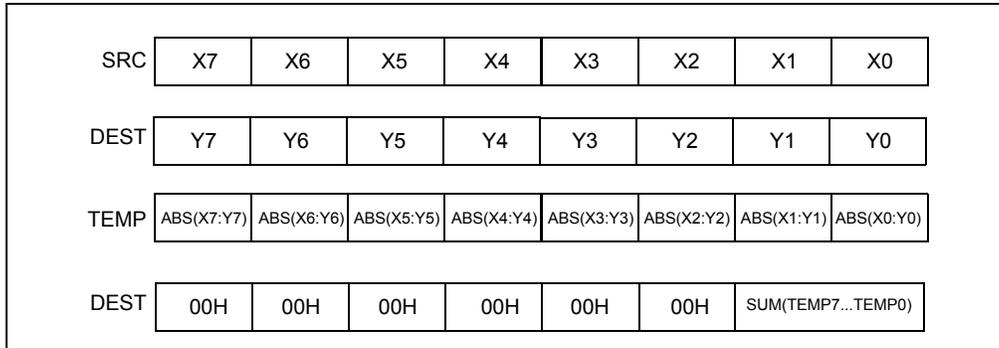
Figure 4-10. PSADBW Instruction Operation Using 64-bit Operands
