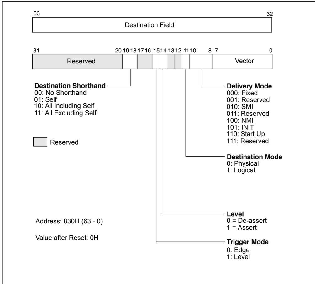
**Figure 10-28. Interrupt Command Register (ICR) in x2APIC Mode**
