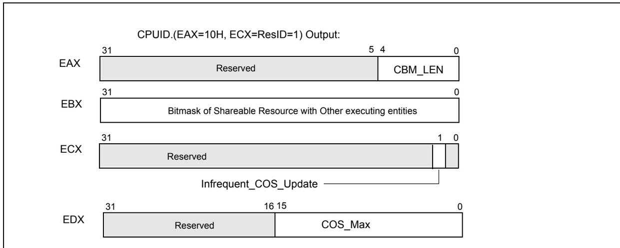
Figure 17-30. L3 Cache QoS Enforcement Enumeration (CPUID.(EAX=10H, ECX=1H) )
