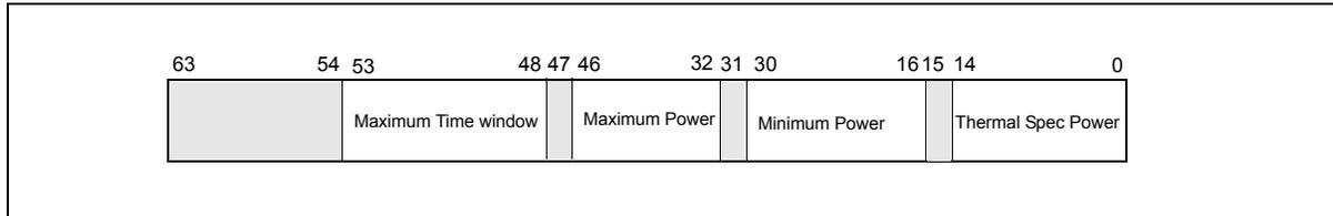
Figure 14-43. MSR\_DRAM\_POWER\_INFO Register
