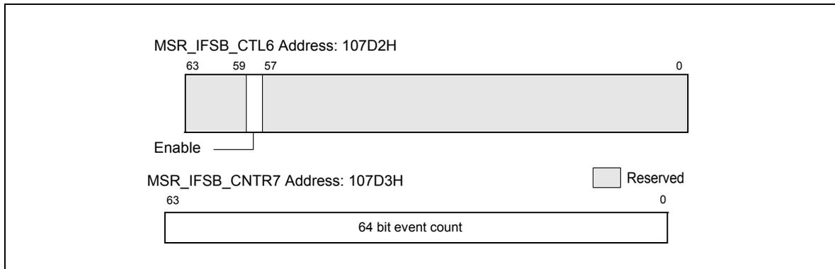
**Figure 18-48. MSR\_IFSB\_CTL6, Address: 107D2H;
