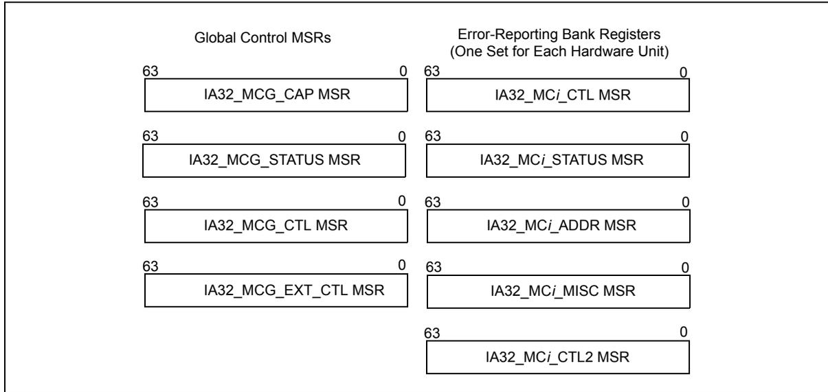
Figure 15-1. Machine-Check MSRs
