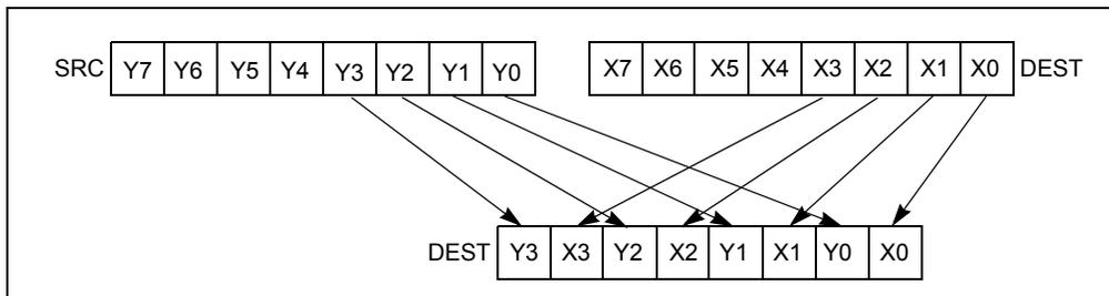
Figure 4-18. PUNPCKLBW Instruction Operation Using 64-bit Operands
