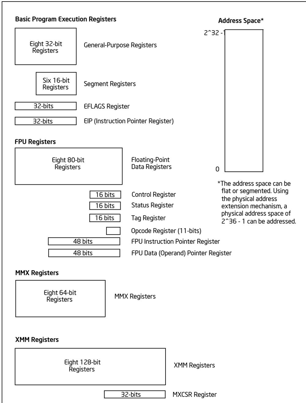
Figure 3-1. IA-32 Basic Execution Environment for Non-64-bit Modes
