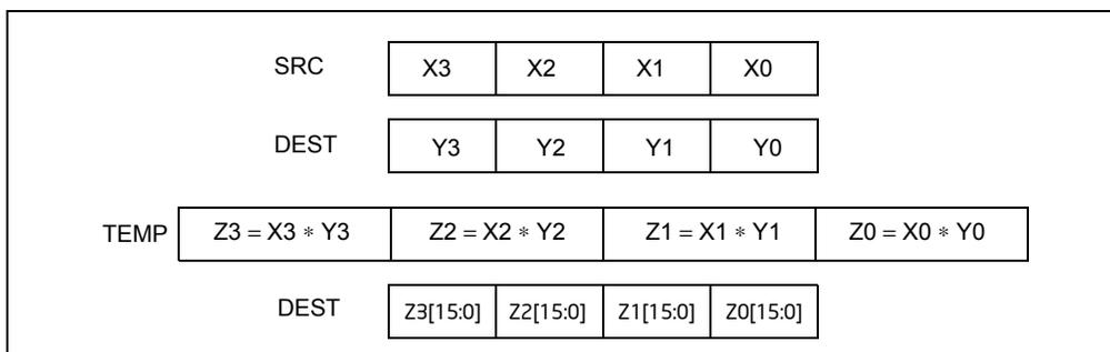
Figure 4-9. PMULLU Instruction Operation Using 64-bit Operands
