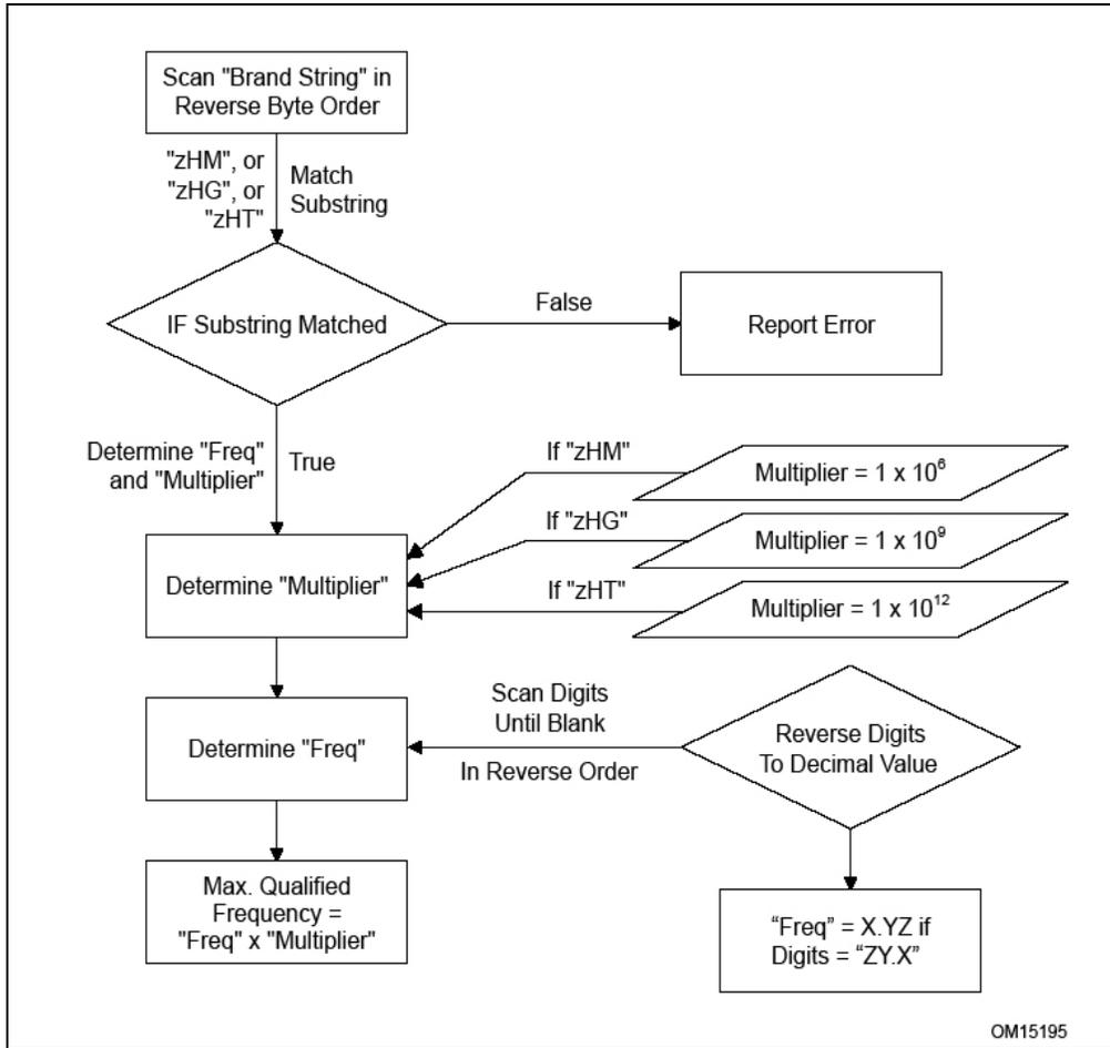
Figure 3-9. Algorithm for Extracting Maximum Processor Frequency
