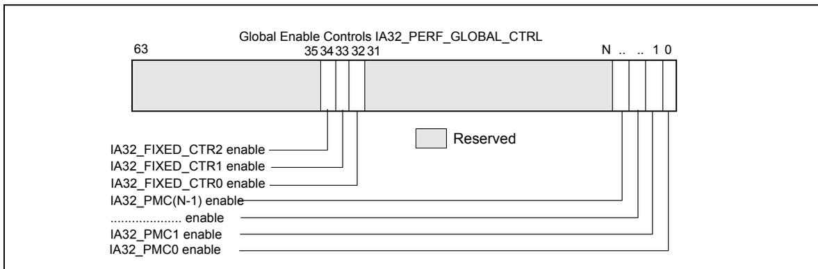
Figure 18-8. Layout of Global Performance Monitoring Control MSR
