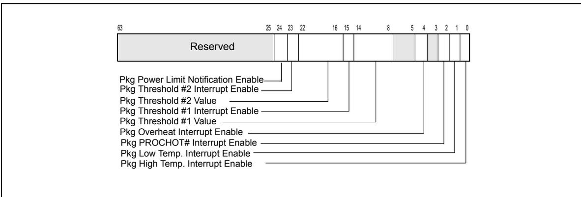
Figure 14-31. IA32\_PACKAGE\_THERM\_INTERRUPT Register
