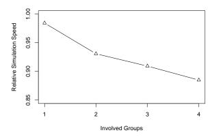
Figure 8: Relative simulation speed of monitoring a coordinated break condition for multiple devices. X-axis is the number of groups (hosts) involved. Y-axis is the ratio to original simulation speed (without condition monitoring).
